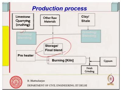
So production process, limestone quarrying and crushing that would be there, other raw materials, so first I think I was mentioning this that you will actually select the quarries based on appropriate composition of limestone and clay, you cannot bring them from different sources and mix, the cost goes higher.
