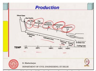
So, this is a production, so this is the kiln, it shows there the burning occurs here, formation of compounds of cement C 3S, C 2S limestone decomposes and sorry, the raw feed comes from there, raw feed comes from there. So this is higher temperature, this is lower temperature, free water will move away. Clay then decomposes, limestone decomposes, C 2S and then C 3S forms, right?
