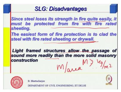
So that slide you know that is what the main problem is fire it must be protected from fire with fire rated sheeting. That is one thing. Protection should clad the steel and fire rated you know fire rated sheeting or drywall. So that is what it is. So passage of sound more readily that is also a problem because sound travels you know (soul) sound (sou) I mean the insulation quality sound insulation quality of steel is not so good.
