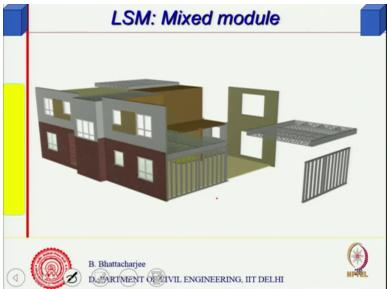
And this is 4 sided open system. So you have just vertical members and there is a floor. So open sided module, completely open sided module. So you can have varieties of module forms and mixed combinations could be there. Judicious use of this combinations can provide good constructions.
