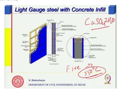
This is what another place is showing, for example, you can have you know pre-crust concrete inside. So you can put you can have pre-crust concrete. So this is your light gauge steel (fra) frame part of the frame and you can have actually or concrete system inside and pre-crust
