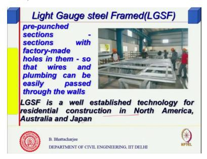
So this is many places in North America, Australia and Japan they have been using this actually. So this is you can have pre-punched sections, sections with factory-made holes so that wires can pass through them, also since is a frame system you can now adjust doors, windows etcetera etcetera you know locally have (())(15:47) those places wherever you want.
