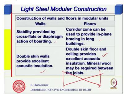
And stability is provided by cross-flats or diaphragm action of the boarding. So corridor zones can be used to provide in-plane bracing in long you know sometime you can have bracings to provide extra stability. Double skin walls provide excellent acoustic insulation as I said and floors also acoustics. You can put in mineral wool or some sort of light weight material which will act as an insulation
