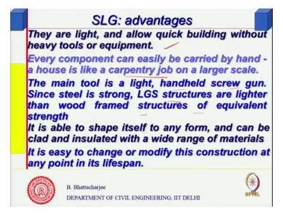
And light allow quick building without heavy tools or equipment. Every component can easily be carried by hand and like you know carpentry. So basically the idea was to replace the timber you know that was the idea. So therefore, we saw all from that side. Generally you need to for
