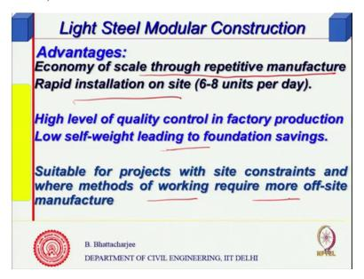
Anyway advantages of light is economy of scale through repetitive manufacture and rapid installations. So that is, then again you need a break-even number because you have to have you know set up factory basically. So high level quality control in factory production and low self-weight leading to foundation saving. Suitable project with site constraints and where methods of working require more off-site manufacture you know its advantages there.
