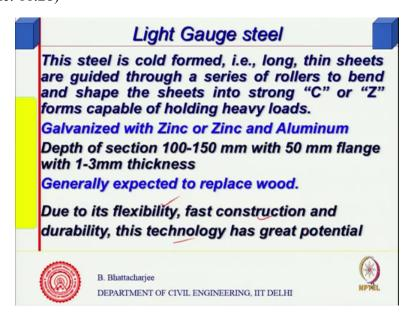
It was actually originally thought of thought to replace wood right it is originally thought to replace wood but because of its flexibility, fast construction and durability so it has got it is quite high potential.
