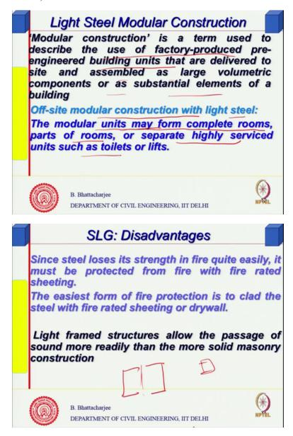
So modular construction so this is you know these issues are acoustic issues are important so what you can do is you can depending upon the situation you can actually introduce. Wherever there is a connection might introduce for example if this is, if there is an issue of acoustic transmission, so between these two might put some other material which is a kind of resilient material and things like that so you have to take care of this.
