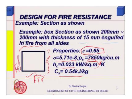
So, we do it in a tabular form for example, consider this section box section let us say I have got 200 mm and 200 mm with thickness of 15 mm engulfed in fire from all sides right. So, this is my steel section engulfed in fire from all sides. So, I have got fire from all sides fire, there is a vertical section let us say it is a column, let us say it is a column I consider 1 meter height.
