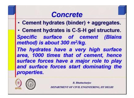
And then we are looking at concrete and we said that cement hydrates, which is the binding material right which holds which goes into the interstices of aggregate system. It is true for asphaltic material also these are actually particulate system bonded together largely, mechanically chemicals are very little chemicals you know chemical bonding is very little.
