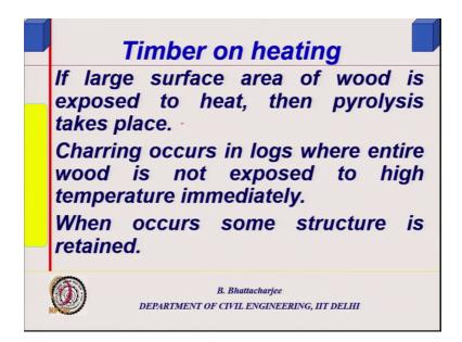
So, if large surface area of wood is exposed to heat then pyrolysis takes place that is what it is. So, charring occurs in logs where entire wood is not exposed to high temperature immediately when occur some structure is retained. (Refer Slide Time: 28:07)
