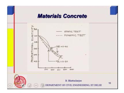
So, that is why you see this kind of behavior and therefore, modulus of elasticity which one would need in design, if somebody is doing a fire design then; you can see that modulus of elasticity relative value it reduces in this manner. Some manner introduces statics tests and dynamics test, what is dynamic test? In dynamic test actually preload it increase the temperature and do it again right?
