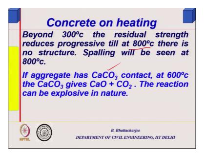
So strength obviously, beyond 300-degree centigrade residual strength reduces and it goes on reducing till 800 degree centigrade, you will be left with very little. And if the aggregate constant contains calcium carbonate that will get disintegrated around 600 degree centigrade if the aggregate is limestone aggregate and that is what I mentioned.
