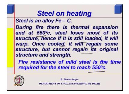
So, steel is an alloy and Fe, Fe and C. There is a thermal expansion up to up to 550 degrees in a thermal expansion, and at 550-degree centigrade steel loses most of it is structure, responsible for strength etcetera, etcetera.
