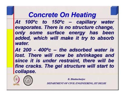
So, that is what I just mentioned in the last class 100 degree centigrade to 150-degree centigrade capillary water will vanish. 200 to 400-degree centigrade adsorbed water will be lost. And this will result in shrinkage and you know cracks etcetera, etcetera due to shrinkage alright.
