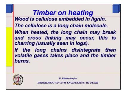
So, timber this is one thing timber shows charring. So, wood is cellulose embedded in lignin. The cellulose is a long chain molecule when heated the long chain may break and
