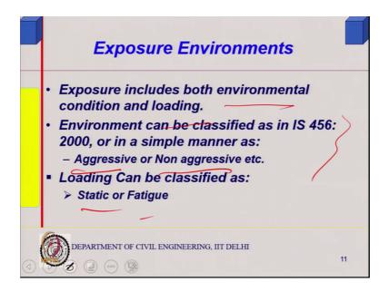
So, exposure environment basically it should include both environmental and loading exposure environment because loading environment is important well things like IS 456 or the prescriptive was do it for durability take care of durability at the beginning, but when you are looking to inspection we simply classify them as aggressive and non aggressive environment and loading static and fatigue because I said the fatigue could be more dangerous.
