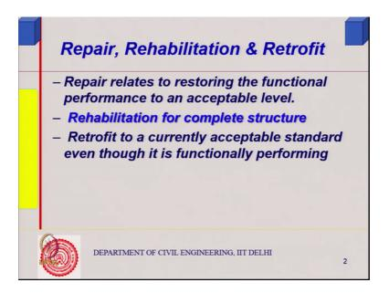
Repair relates to restoring the functional performance to an acceptable level that is what we defined earlier. Also and we talk in terms of patch repairs small areas repair rehabilitation is for the rehabilitation is for the rehabilitation is for the complete structures.
