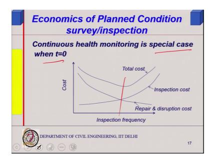
That model needs that kind of a model would need actually finding out the rate of deterioration. So, inspection cost increases in this manner repair and disruption cost will decrease there is an optimal point, but quantifying them is still a challenge at the moment you know quantify how much deterioration will occur at what time is the challenge if you know that then you can easily model this.
