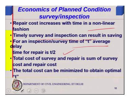
So, repair cost increases with time in non-linear manner cost was increasing in non-linear manner and timely survey and inspection can result in saving.
