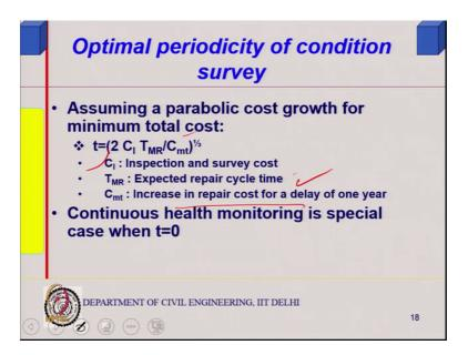
So, one can model this as a I saying, but then the T MRs is expected repair cycle time one can model this actually from those cost curves, but you going to know optimal you know and also rate at which actually the C mt is the increase of repair cost for a delay of one year this kind of model. One can obtain right t is the optimal inspection time you can simply write the equation and differentiate it.
