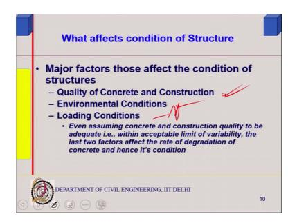
Now, obviously the quality is very important that is what we have seen. So, far environmental condition also loading condition is important loading condition is important because of fatigue loading one will be more susceptible to damages rather than where you have static load.
