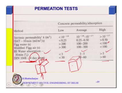
I described there is another BS absorption test what you do you cut a 75 mm core and put it in an absorption tests must in distilled water for half an hour in some standardized procedure the amount of absorption. If it is high, it is a bad concrete high permeably high permeability moderate permeability and low permeability. So, this way it can be classified.
