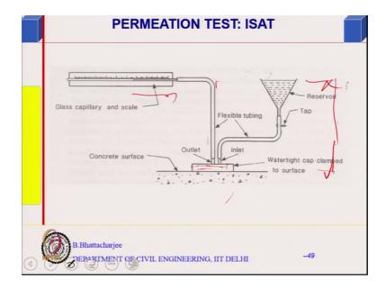
It is a British code test what you do is you have a constant head reservoir right 200 is 200 mm 20 centimetre. So, nothing, but a panel and there is a pipe now there is you know you can close it. There is a clip or tap here which can close this is this is a kind of a watertight clamped to surface right. So, this gets filled with water to start with and this is same height as this in there is a capillary tube where any flow of concrete flow of water can be measured.
