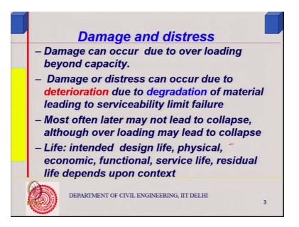
Damage can occur due to loading beyond capacity damage or distress can occur due to deterioration or degradation of material leading to serviceability limit failure right. So, this can occur over a long period of time.
