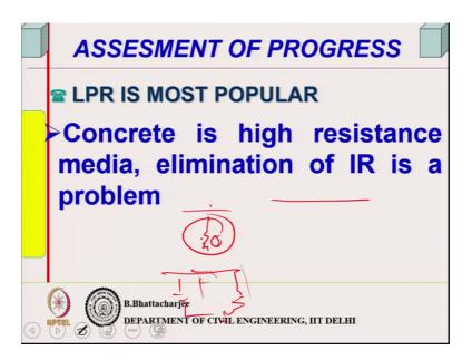
But concrete resistance is very high. So, the resistance that I have showing from the concrete surface to this is very high. So, this has to be eliminated because, polarization resistance is only at the interface, polarization resistance is only at the interface. You know, so this is what I am saying, there is a capacitor and there is another resistance, so equivalent resistance of this part is polarization resistance.
