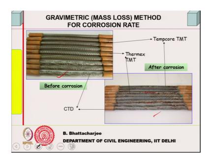
This is before corrosion, after corrosion, bar will look like this. You can say this is corroded, this is corroded right. Then you wash it off and find out the original mass is known to you, you find out the remaining mass. And if you found out the area here then you can find the corrosion current density.
