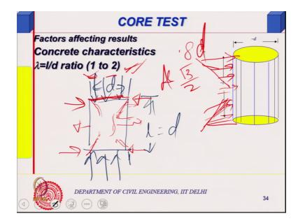
So, l is the length, d is the diameter and you know, factors you have seen factors affect the result is l by d right. Obviously concrete characteristics will effect, but l by d, l by d ratio is important. Now why l by d ratio is important? You know, the strength of cube is more than that of the cylinder, strength of cube because the reason is when you are testing uniaxially a cylinder let us say l; which is equals to d and this is equals to d.
