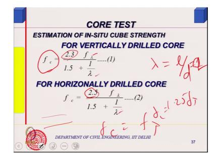
And this is the, you know, estimation of in-situ strength. What you measure is a strength of the sample, from that I should be able to predict the in-situ strength or equivalent cube strength.
