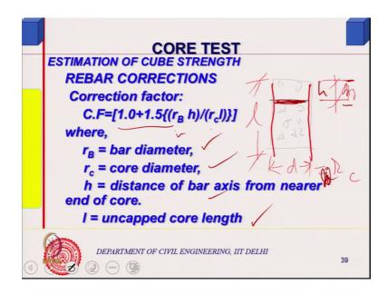
So, reinforcement correction is given like this. You have say, this is your core, l is there, d is there and you have a reinforcement, you have a reinforcement here; which is at a distance h from the nearest place this is h. So, this distance is h from the nearest place.
