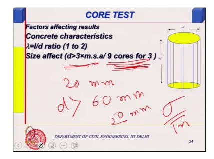
So, I by d has an effect, I by d has an has effect on the strength, size affect as I said so, minimum d is should be 3 times the m s a. Minimum d should be 3 times the m s a, right? Because then if it is nano size maximum size of aggregate. Supposing you was using 20 mm aggregate that is d should be greater than 60 mm. Then you are getting a
