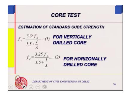
Vertically drilled core is this, and horizontally drilled core is something like this. So, this is this layer effects are taken into account there. The multiplying factor is there is a fractional, you know, this is around 0.8 times, 8 percent difference. So, you can see that 2.5 into 0.92 or so will give you 2.3. So, that affect is taken into account for vertically drilled core and horizontally drilled core.
