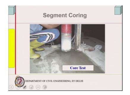
Now, you can see this is the drilling machine, this is the drilling you know, this is the drilling machine the coring is done. So, with a rotary drill this is a bit diamond bit.
