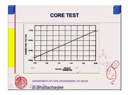
So, 1 by d equals to 2 this value is 1; that means, you have finding same as cylinder strength. L by d is equals to 1, multiplying factor is 0.88. So, you first you find out the equivalent cylinder strength. So, this is a correction factor which you find out from big for u r l by d for u r l by d, find out what is the correction factor.
