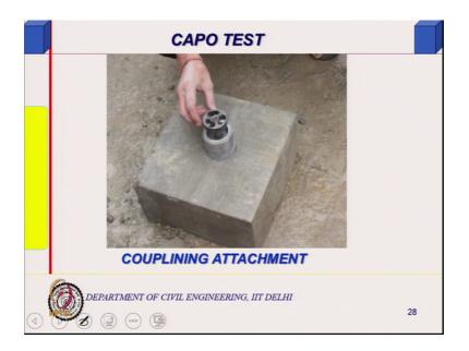
So, placing it and then placing the inserts and pull off test also we did.
