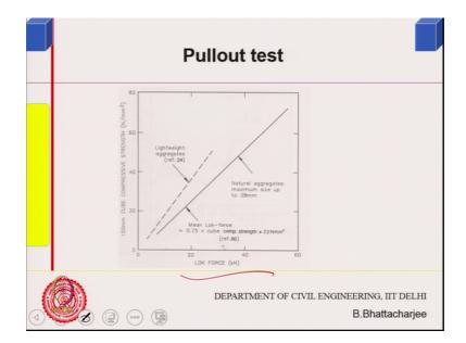
You know, so, basically correlation can be established the force required to pull out force required to pull out is a measure of the compressive strength. So, some sort of correlation with 150 mm cube one can get with different types of aggregate and this are the available.
