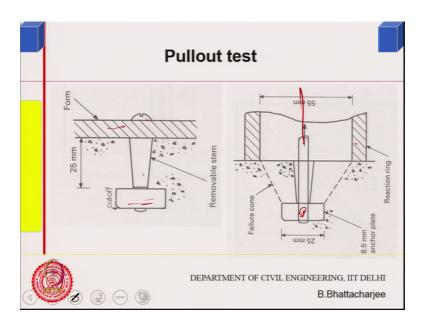
This is a insert that you are putting this is our form work this is threaded and this insert has gone right in the beginning right and then after the concrete has partially set, you know before final setting you just unscrew it and take it out.
