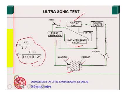
I suppose, I have a diagram. Yes, it will looks something like this. I will come back to that slide later on. So, you have a transducer and a receiver. Now, this transducer is connected to a pulse generator which will generate the ultrasonic pulses, you know some sort of oscillator and then converts this electrical energy into mechanical waves right.
