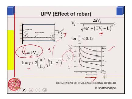
So, rebar effect is important effect of rebar if it is along the direction then you need some corrections which would actually because it will travel through this. So, velocity in steel then becomes important. So, if you know because it will travel through this path. So, correction is needed velocity has to be corrected using this kind of a formula where a you know this is this a length this length is a.
