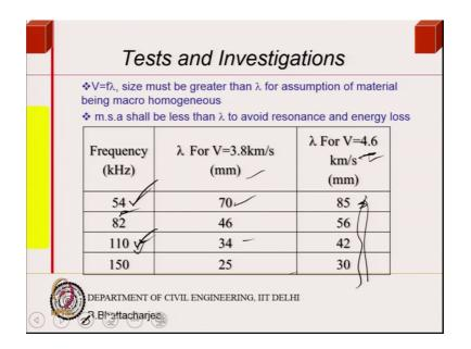
Now, V is equals to f into lambda velocity into frequency. So, size must be greater than lambda that is what I said for assumption of material be macro homogenous right. It should be homogeneous because I am assuming concrete to be homogeneous and m s a shall be less than lambda to avoid resonance and energy loss.
