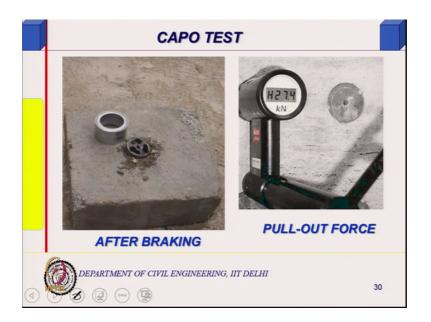
And this is you know, this is how after breaking you get some sort of thing this is the machine where you read how much kilo Newton is a pull out force from here it came out.
