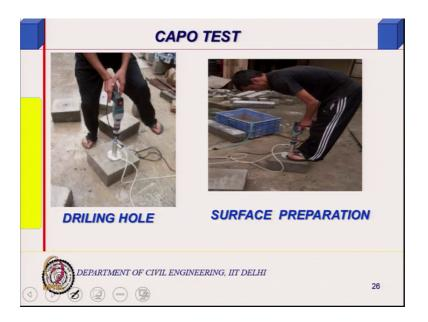
Drilling hole surface preparation.
