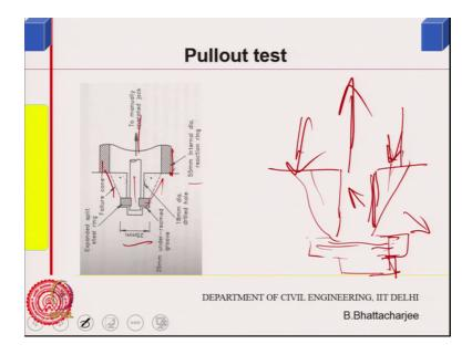
What it does it? You drill a small hole into the concrete right. So, this your concrete surface you drill a small hole and the instrument is there which can actually cut a group likes thing. It can cut a group cut a group, it can cut a group, it can cut a group into the concrete and this pull out device, it will have a kind of flangia here right, then this is pulled out with the reaction taken you press it from top press it here and pull out here press it here and pull out here.
