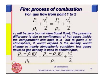
So, we look at the Process of combustion; repeat some of the portions what we have done last time. We have seen that we can apply Bernoullis equation to point 1, 2 and 3, 4. And since there is no no bulk movement, you know there is there is no streamline flow at 1, so we take v 1 equals to 0, and v 2 because that was at the top v 1 is inside, and v 2 is just outside at the hot gases. And v 2 is what we are interested in finding, so that we can quantify the quantity of volume of flow.
