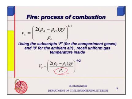
So, so that is how we do it. So, rho 4 is rho F right. So, putting F and 0 subscript that is what we get overall it is rho 0 because hot cold air, air is coming in and that is how we get the velocity at a distance y below the neutral axis of fresh air right.
