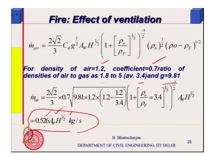
So, so C d appropriate value of C d, so by doing all this you know one can actually find out for density of air to be 1.2; C d is equals to 0.7, ratio of densities so take three point yeah four is averaged; g 9.81. By doing all this, for wood actually one can get a value of 0.526 A W H to the power half. What is important to understand is that it is a function of this factor, ventilation factor a constant multiplied by ventilation factor.
