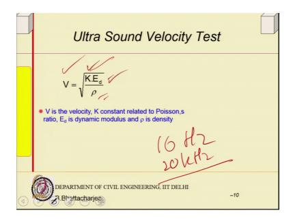
You can you an derive this. You can derive this because mechanical wave velocity of mechanical wave not sound I mean ultrasound or whatever it is velocity of mechanical wave, after all we know that longitudinal wave is nothing but compression and tension of the you know it is compression rarefaction of the material or medium. So, if it is passing through the concrete it must be compressing the concrete and must be it must be expanding and compressing and expanding and compressing.
