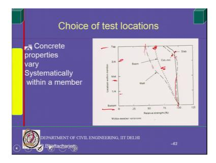
Then test locations now, I said concrete strength varies systematically in concrete. For example, if you see typically for a column strength at the bottom is if I assume it to be 100 percent 1 percent variation is much less than the top. So this is top, this is bottom, this is mid height three fourth height one fourth height etcetera etcetera.
