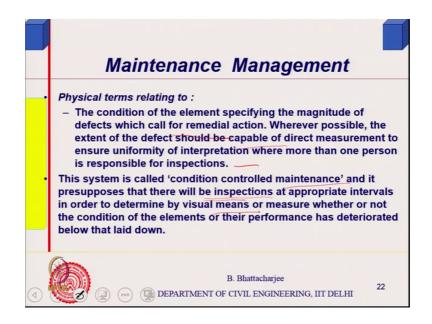
So, one is physical term simply physical term measurable item right: The condition of the element specifying the magnitude of defects, which will require remedial action alright. Wherever possible the extent of the defect should be capable of direct measurement right, to ensure uniformity of interpretation where more than one person is responsible for inspection. As usual say later on a plan maintenance would invariably I mean; it must it is a you know inspection is a must for plan maintenance.
