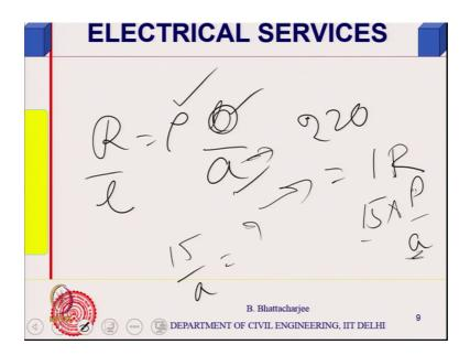
For example is pretty simple, Cable capacity you want to calculate out, we know that resistance is equals to rho into l over a.
