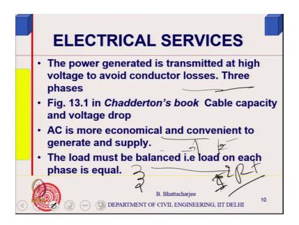
The other issue is important, the power generated why alternating currents are used actually. The power generated is transmitted at high voltage to avoid conductor losses. Very high voltage, low current right so three phase generation is easier, transmission is easier. Cable capacity you can calculate out very easily, but this (Refer Time: 22:32) also.
