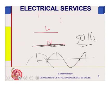
So, in a single phase supply, you have two wires live and neutral, usually this is black this is black, this is red, usually this is black, and this is red. Now, we know that our supply voltage is sinusoidal right sinusoidal. So, single phase means, I have with 50 hertz frequency sinusoidal voltage. Three phase means, I will have three phases, which will be 120 degree out of phase peak to peak would be 120 degree means, 360 is a complete cycle from starting from here to here.
