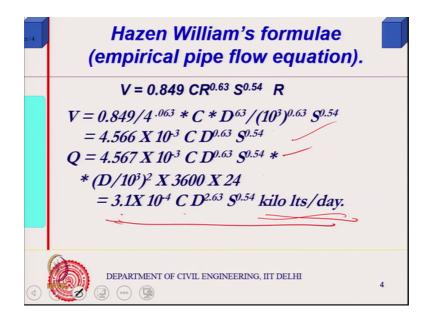
Perimeter you know like equator perimeter and those. And then flow is equals to I must multiply by area right. So, V is equals to and the units are very very much important, units are very much important. So, this was in you know this you have to convert into appropriate unit, so that is why if D is in millimeter, you want to converted into meter right 10 to the power 3 0.63 again comes in. And this is also, because D to the power, you know this, if I look at this R is A by P which is D by 4.
