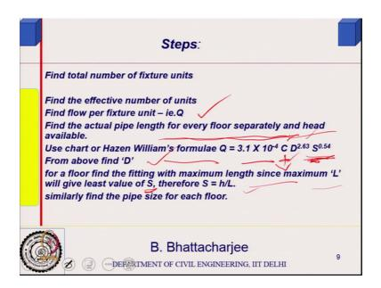
So, if you know that once you know the number of fixture units, once you know the total number of fixture units and effective fixture units, flow of per fixture unit you know is Q then Q multiplied by, you know flow per fixture unit is given Q which I will just tell you in a minute, in a minute I will just tell you. So, then you can find out the total flow, because multiplied by the effective number of fixture unit by Q. In fact, they give you another chart or table also is also available.
