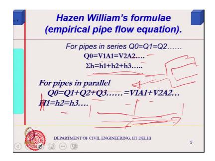
So, a consider now pipes in series. Then flow is constant there are some basic equations actually research will look into some basic equation. Then look into the actual building and things like that. So, V 1 A 1 must be equals to V 2 right. Supposing the 2 pipes there is one pipe and there is in another pipe. And this pipes are in series flow must be constant, if it is a study flow flows you know flows constant.
