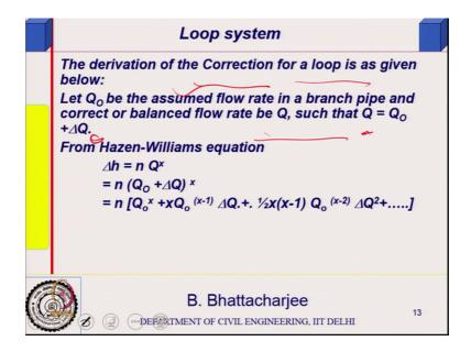
So, what is done basic equation is something like this. You have to first assume find out the sigma h f value in a loop that should be equals to 0 if not 0 that is the error. So, this derivation of the you know correction, you have to do a; you have to do a correction for the same, you have to do a correction for the same right. So, we will just do that. You derive this formula for this one. For example, Q 0 may be assumed flow rate in a branch
