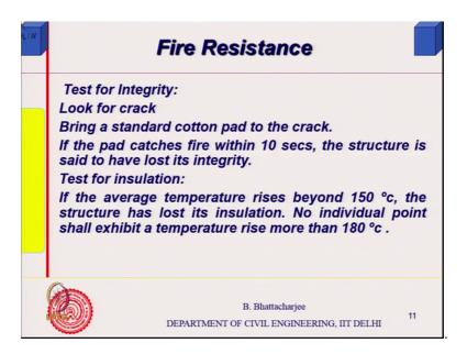
So, that is how we test for integrity, test for insulation we look for temperature rise on the other side. So, here we are now looking average temperature if it goes beyond 150 degree centigrade, then the structure is lost his insulation quality. And no individual point shall exhibit a temperature rise more than 180 degree centigrade.
