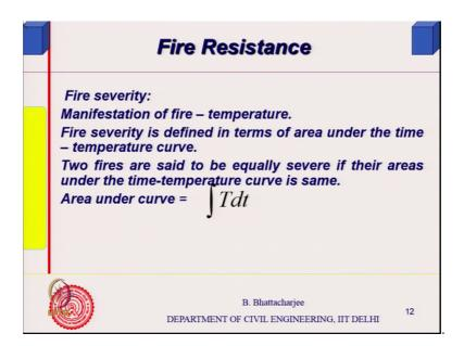
So, the area under the curve has to be same. So, area under curve will be integral capital T is temperature dt is the time small t is the time. So, integral T dt should be same right integral T is T dt will be same.
