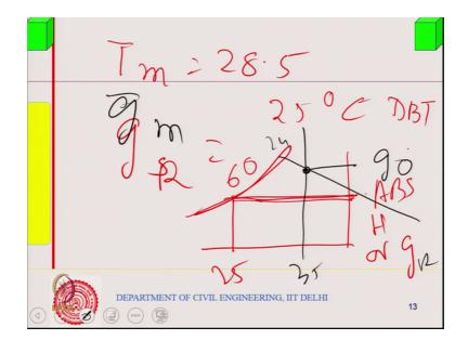
So, temperature of the mixture we have seen that T m is equals to 28.5, g of the supply g of the, you know mixture I have to find out. But first groom room moisture content of the room will correspond to DBT 25, DBT sorry 25 degree centigrade DBT. And how much is a wet bulb temperature? Is given or.
