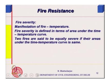
If I have defined them somewhere ok. So, fire load is that is how we define fire load. Now, I if I have to compare a building element, you have to compare a building element for its performance against fire, I must have some way to quantify this performance right and from this point of the point of view what it would be for example, if it is a wall or a you know roof or ceiling floor slab or the floor system floor system a floor, then I must be able to quantify their fire performance.
