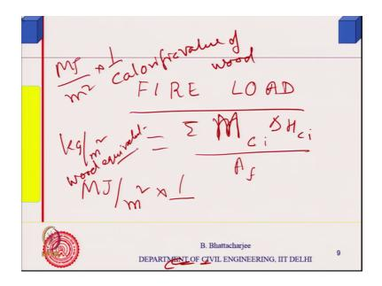
We define in terms of fire load. Now, what is fire load? Fire load is you can identify total quantity of combustible material in the room, total quantity of combustible material in the room divided by the area floor area or internal surface area you know people use both this, but generally it is floor area right. So, fire load is nothing but sum total of all combustible material multiplied by their delta h c. So, it would be actually mass, mass right mass of the combustible material.
