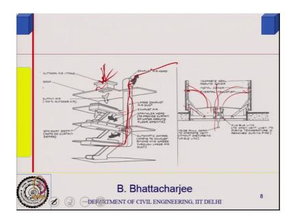
Typical smoke vents would look and vertical smoke vents can look like this is normally in closed position like this, right; held up by sort of a string, but supported in this manner. As soon as the fire breaks out, the few link that holds it in position breaks and it can go open up in this manner allowing smoke to go out.
