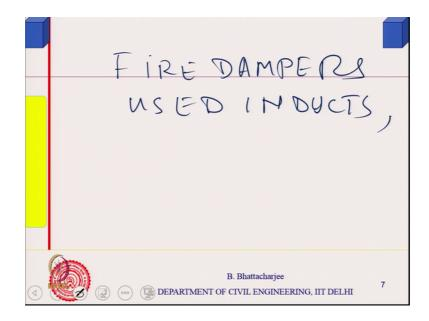
So, fire dampers were one issue fire dampers as I said, fire dampers fire dampers these are used in ducts used in ducts and in case of fire, they do not allow and an along a transmission of hot gases, etcetera, etcetera. So, essentially also you do a kind of insulation lining around the entry point. So, that the heat also hot you know the
