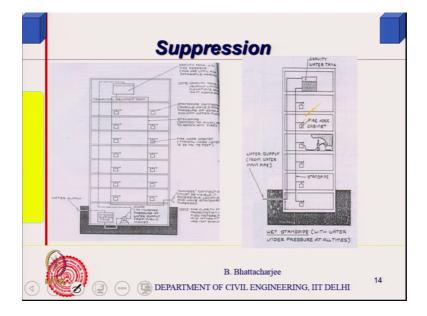
So, now, you can have combination you can have combinations for example, we can have a wet riser as well as you know you can have wet riser as well as dry pipe systems of this is your dry.
