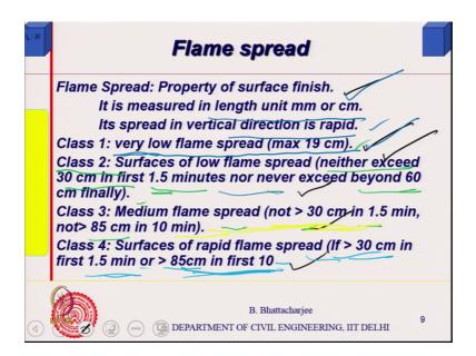
So, 4 classes of flame spread finishings is essentially related to finishing surface finish right. So, it is the property of surface finish actually property of surface finish property of surface finish right. So, this is the; and its unit is millimeter or centimeter in length unit right now we can talk in terms of rate of spread. So, rapid flame spread usually vertical flame spread is faster so, but there can be situations where it is horizontal space more.
