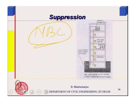
So, this was a wet pipe system you have a tank and this is always water is under pressure if this is the pipe, this is the wet wipe you know on which water is under a pressure.
