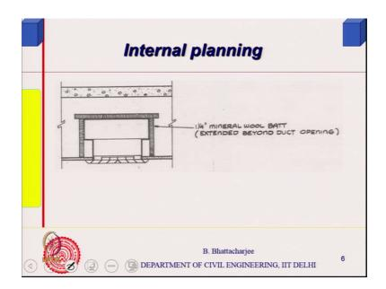
You might have insulations here. For example: you can have a insulations mineral wool insulations, mineral wool insulations, etcetera, etcetera, so that you know heat is not transmitted to the duct thermally thermal heat transfer is minimized. So, this is one issue.
