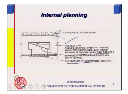
For example, we can have something like this as I said is a fusible link, you know and holds the damper open at normal room temperature, but melts releasing damper and you can have damper with a asbestos or insulation on both the sides. So, this is the fusible link which holds it and just it melts and then it can come or in some manner, it has to support essentially, it will be supported from the top, because that that is why it can hold it.
