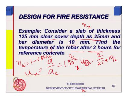
Simple case, of thickness 125 mm, thickness of the slab, cover depth is 25 mm and bar diameter is 10 mm. Clear cover depth is 25 mm.
