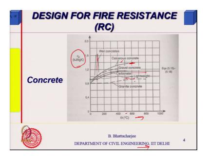
So, properties if you look at it, how does properties very thermal conductivity? For example, sorry specific heat for example increases and say a function of type of aggregate. Yes, temperature function of temperature and with temperature it also depends upon aggregate. Wet concrete of course, has got a very high specific heat, because wet concrete means water.
