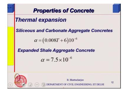
Expansion is again property is increases with temperature. And shale aggregate as I shown the earlier diagram. So, this how it is.
