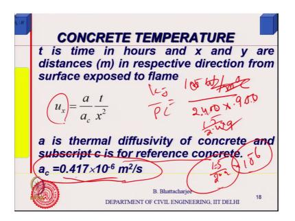
Now a is the thermal diffusivity the concrete that your concrete. And subscript c is for some reference concrete which is constant. So, reference concrete value is taken as 0.417 10 to the power minus 6 meter square per second, right.
