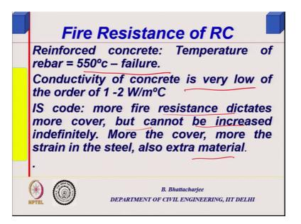
So, that is you know again we assume the reinforced concrete temperature of rebar is 550 degree centigrade at failure; 550 degree centigrade at failure. Conductivity of concrete is very low 1 to 2. And the as I told you more fire resistance dictates more cover, but cannot be increased infinitely or indefinitely. More the cover more the strain in the steel also extra material, so, cost will increase.
