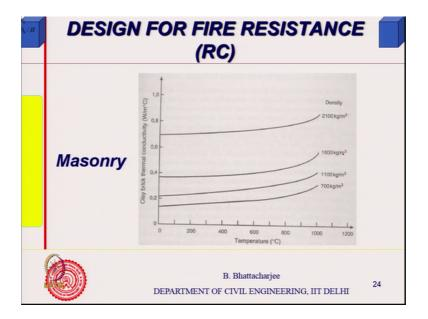
And the same brick thermal conductivity is of this kind, not much studies are available on brick. So, that is what it is. So, having looked at the having looked at the fire resistance concepts and design of structural member, some members not structural, it could be for non-structural members also; for, you know, fire resistance design for fire resistance from thermal point of view.
