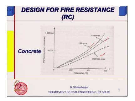
Thermal expansion, it increases depending upon type of aggregate shales, siliceous, carbonate aggregate etcetera.
