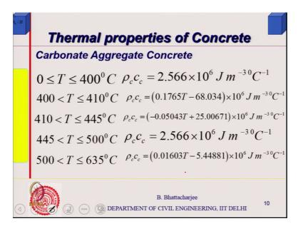
So, for carbonate aggregate the formulas are different, formula is somewhat different, but there similar nature and similar results are available. I again do not expect you to remember, but you understand that is a function of temperature and step functions. In fact, it is not cannot be defined by a single functions.
