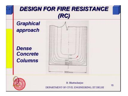
For column or beam members temperature contours are given, right. Temperature contours are given. So, this is for example, 100 degree centigrade, 200 degree centigrade at a given time. So, similar graphs are available for various times, right. So, supposing you know the cover depth, right. This is given at as I said at different times. The time at which that the cover depth this temperature reaches 550, you can find out the corner steel and so on.
