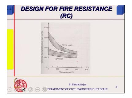
So, the some other results normal weight concrete, light weight concrete, that is a kind of band. So, lightweight concrete it does not change much thermal conductivity, but for normal weight concrete conductivity changes with temperature, reduces down.
