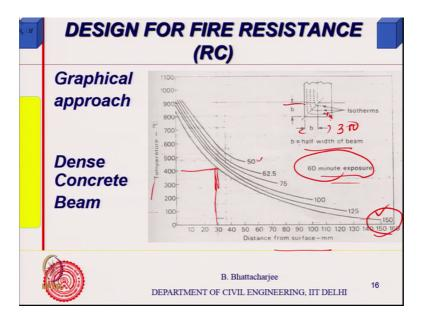
As I said for each time there is one set of graph. So, 60 minute exposure right this is 50 degree centigrade, ok. And 150 degree centigrade etcetera etcetrea distance from the surface. So, distance from the surface 30 say let us say 30 mm, distance from the surface wherever it is corner steel you will consider the diagonal distance.
