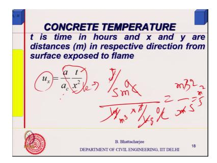
What is joules per second? So, conductivity unit is this, conductivity k unit is this joules per second which is what meter degree centigrade right. And specific rho is kg per meter cube multiplied by joules per kg per degree centigrade.
