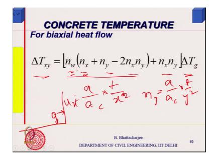
You can find out and find out the temperature, when it becomes 550 t you can in find out corresponding to 550. And that would give you the fire resistance.
