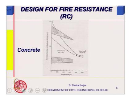
For this I will just give you thermal conductivity lightweight aggregate concrete, it is nearly constant over a bend.
