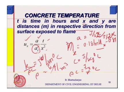
So, t is the time in hours. Now since the empirical, the unit is very important, t is the time in hours, x and y are distances in respective direction from exposed surface; u x that was I just talked about, because I said that n x n x is equals to, you know, it was how much? n x is equals to 0.8 right. So, 0.18 ln u x minus.
