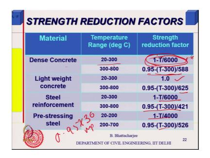
This can be used in residual post fire residual evaluation as well. So, 20 to 300 degree centigrade for dense concrete, it is taken as approximately strength reduction factor is taken. So, this reduction factor is less than 1. If the concrete strength mean strength let us say is 30 multiplied by this factor. Say 200, if 3 is equals to 200 or 300, let us say T is equals to 300, how much will this value we? 300 by 6000, so, it is 0.5,
