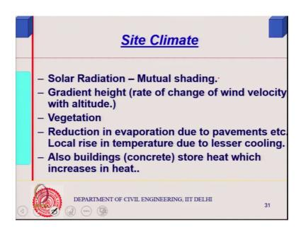
Gradient height as we said you know temperature I mean velocity wind velocity it increases with the height and radiant height changes. Topography if it is all rough gradient height is more if it is plain radiant height is.
