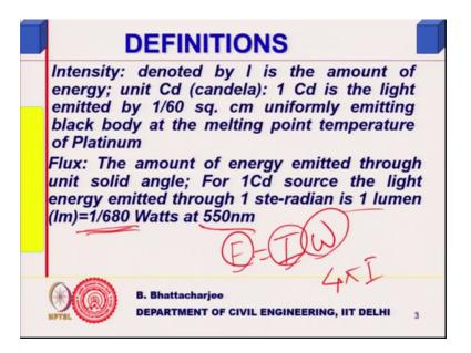
So, that is the definition of lumen or unit you know that unit and just compare this with watts 1 lumen is equals to 1 by 680 lumen you know sorry 680 watts 1 by 680 watts.
