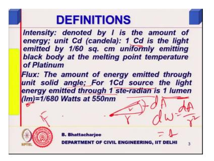
We talk in terms of energy emitted through you need solid angle, for 1 candela source the light energy emitted through one ste radian, you know you remember we talked of solid angle earlier. So, 4 pi ste radian is the solid angle subtended at a point you know in all direction of spherical front going on.
