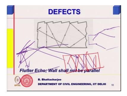
When you even your parallel, you know when you have parallel for example, this is your parallel wall. So, what will happen, it will reflected wave will travel like this and the other reflected wave other reflected wave might travel in like this, this causes a fluttering sort of an effect. So, when your parallel wall close to the proscenium or stage source they tend to cause a reflection back and forth, parallel walls because angle of incident will be small. So, will be the angle of reflection.
