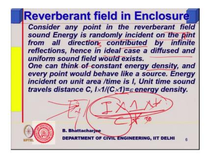
Now any point in the reverberant field basically if I consider in the whole volume of the room enclosure. So, it would receive I am keeping the direct sound out only the reflected sound and infinite reflections will reach to any point like that is what we have seen through this diagram if you recollect.
