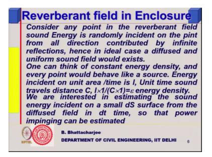
Our interest actually estimating the our interest is to estimate the sound energy incident on any surface I am assumed from the reverberant field, the reverberant field I can treat it as a point source right treat it as a point source every point and from that how much is the energy incident onto the different walls, why I am interested because some of this energy will come back, some energy will be absorbed by the surface itself.
