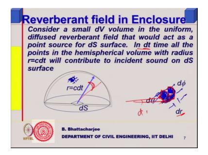
I am using is the energy in that small dV volume. So, dV volume let me consider and that would act as a point source for dS surface right in dt time all the points in the hemispherical how much no supposing I consider a surface like this surface like this said this is my dS surface. So, this is my dS surface this is my dS surface.
