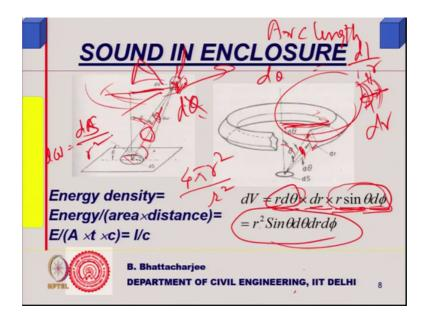
So, this is what I was trying to do in the last class energy density is I by c I take a small volume there dV and I said that dV can be written as rd theta because this angle is theta right and it makes an angle of d theta here this angle is theta. So, this, this normal to the surface and this point is theta and I am calling this, this covering it d theta this part is d theta.
