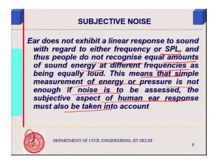
So, therefore, ear does not exhibit linear response to intensity right, which either frequency or sound pressure level or intensity whatever we call it and thus people do not recognize equal amounts of sound energy at different frequencies.
