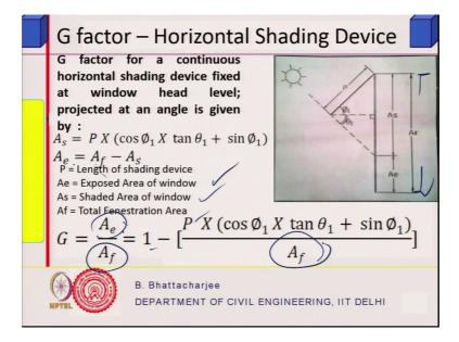
So, G factor is continuous horizontal for a continuous horizontal shading was fixed at window head level projected at an angle is given by this, A e is equals to total is A f total fenestration height or area is A f minus A s is A e is what is receiving the radiation that multiplied by intensity of radiation in that particular time, both are function of time you can sum it up for the whole year. So, P is the length of the shading device, e is exposed area, shaded window, total is this.
