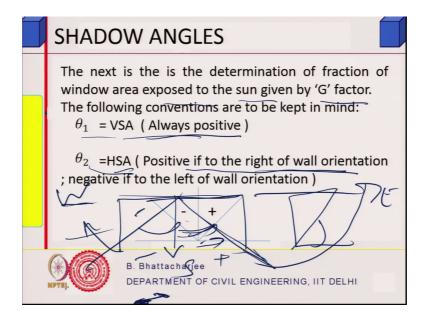
So, the next is the determination of fraction of window area exposed to the sun given by a factor G vertical shadow angle is always positive because it is like that right it. So, it will be always positive vertical shadow, will always positive it cannot be negative because it is from the horizontal ground to vertically upward touching the touching the tip of the shading device, right.
