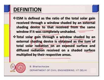
So, you can see the similarity it is the solar gain solar gain received through the window shaded by an external shading device to that received from the same window if it was completely unshaded, right. So, it is the ratio actually.
