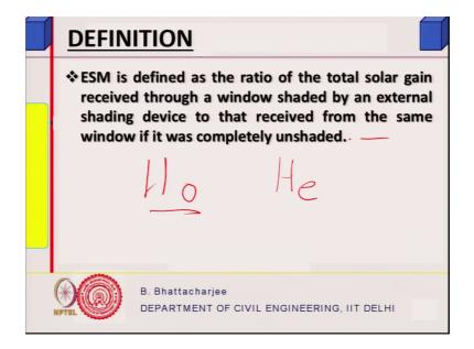
So, external shading multiplier is defined as a ratio of the total solar gain received through a window shaded by an external shading device to that received from the same window if it was completely unshaded. Now, remember H o you must be remembering sometime I talk to about H o right H o was the that is right you know we defined we used something like H o then used H e etcetera. What was H o?
