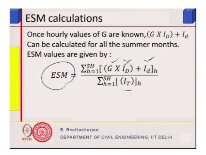
So, external shading multiplied is G and I direct and if we have diffused which will come from half of the hemisphere, diffused to which will come from half of the hemisphere because vertical one it sees does not see the full hemisphere, only one side supposing it is facing south. So, it will see two quadrants south eastern and south west so, total diffuse sky radiation is known half of it can be taken.
