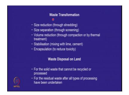
After this we may want to we may still have some waste left and we might want to transform the waste. For example, you might want to shred the waste to make it into smaller you have large sized waste, you can shred it or you can grind it. You can do size separation through screening, mixed waste is coming to you to a site, you do screening. The waste which is more than what is the signs, how many mm is this or how many centimeters of this?
