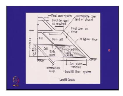
And also we looked at how the waste is placed in daily cells with daily covers and finally, a final cover system.
