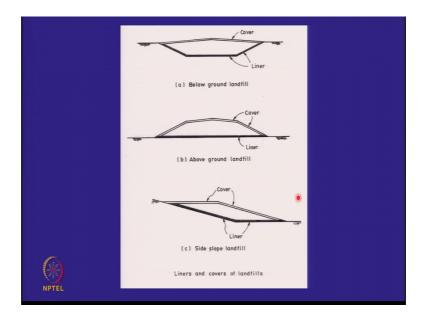
And we recognized there are different shapes and sizes of landfills and we talked about below ground landfills above ground landfills and site slope landfills.
