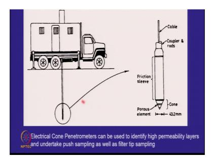
So, in contaminated sites we talked about high end equipment which can be pushed into the ground of the electrical cone with the filter tip.
