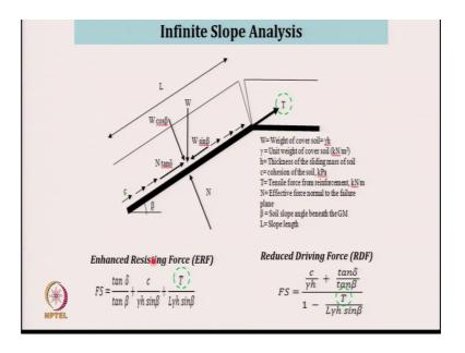
We were we recognize that one of the critical aspects is the failure of the soil or sloping surfaces above the geomembrane and how this was often found to slip and we had to take adequate measures.
