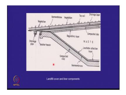
Gradually we developed the concept of multi layered system for the covers and for the liners and we started to look at what a landfill actually looks like in section.
