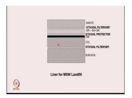
And how it In fact, was not one layer or a 2 layer system, but several layers with separators and protectors and filters and the composite barrier being the key component of the liner system.
