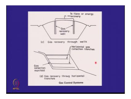
We also discussed how we collect gas through active systems and passive systems and through wells and through horizontal collection pipes.
