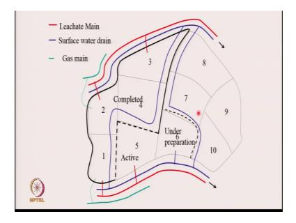
Then we looked at the fact that a landfill cannot be constructed in one go, but for you have to construct it in phases. So, example here is the landfill, which is constructed in 10 years. And how every year you complete and close a phase, there is an active phase and there is an under preparation phase and how the surface water drainage systems the leachate collection systems the gas collection systems have to be developed as the landfill moves forward year by year.
