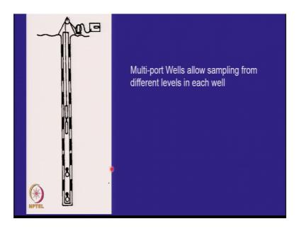
That means, in one well how you can take samples from different depths.
