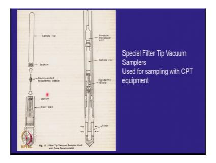
And how we can also use a special vacuum samplers to take out this and detect what is the contamination at various depths.
