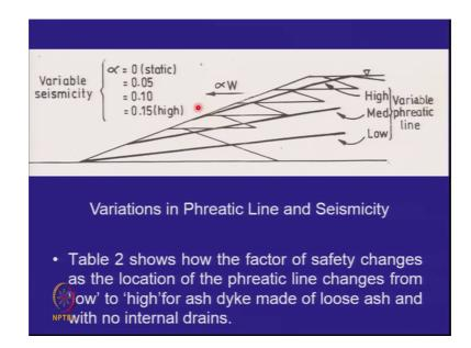
So, here is the first set of variables. What is stated is you could have a high phreatic line, a medium level phreatic line and a low phreatic line. When will the phreatic line will be low when the pond is of low height ashes just filled up a meter or 2, and the water is one
