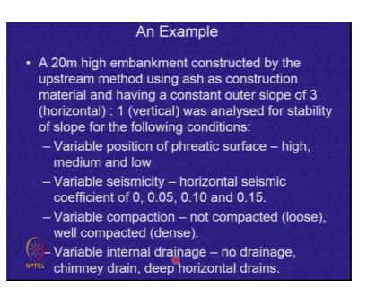
So, I am going to take an example and show you how various parameters effects the stability of embankments constructed by the upstream method. A 20 meter high embankment has been constructed, the outer slope has been kept three horizontal to one vertical. And we have varied the phreatic line, we have varied the horizontal seismic coefficient, and we have varied the compaction as well as the internal drainage, so that is the problem that has been analyzed.
