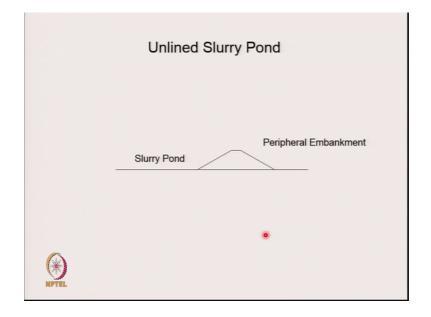
So, let us say this is my slurry pond this is the peripheral embankment earlier it was unlined right. And what use to happen you would have your ash and slurry water up to this point and then I had to make the next raising. So, I would stop one portion of my pond from working and do my discharge in the other portion.
