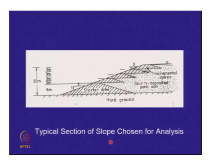
Please note that his is first starter dyke is 8 meters high, and here are 1, 2, 3, 4 reasons of 3 meters, the downstream slope is 3 is tau 1. And there is no offset at the level of the crest. Normally, you may have this kind of a construction or many times you move the upstream dyke a little behind and leave a 2 to 3 meter wide pathway, so that that can become an inspection path.
