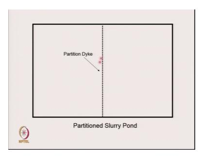
So, I do the partition I do a partition dyke, now I have two ponds. One can be working at one time, the other can be closed the other can be working at one time the first one can be closed and I tend to keep the decantation wells close to the embankment.
