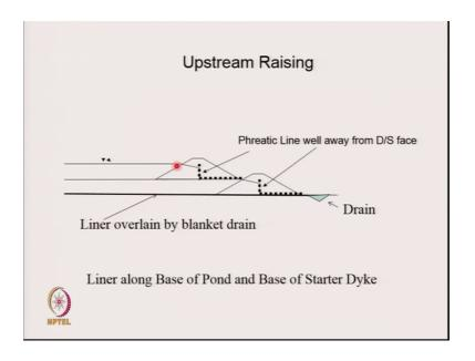
Consequently if you look at the options, so here you see that here what they have done is they have taken the liner overlain by a blanket drain through the dyke. And they have therefore, allowed the water to collect at the drain. In such a case, the ponded water would come down and you would be able to collect make your first raising with no problems.
