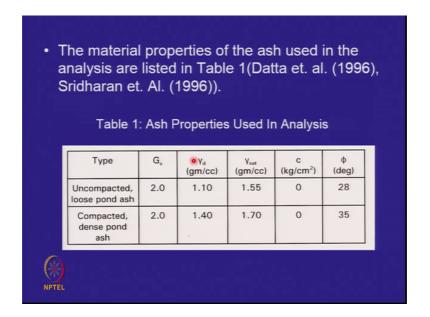
Way we used this analysis for an ash pond. So, the properties of the ash for loose uncompacted ash, this is hydraulically deposited and compacted ash which is compacted by rollers were taken. The important thing to notice is that the phi dash for the hydraulically deposited ash was taken as 28 and for the compacted ash was taken as 35.
