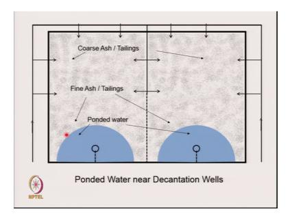
So, let us look at this I will have coarse action tailings very close to all these area, but I will have fine ash and tailings here. So, what happens I have to raise this now by the upstream method. The upstream method means my new dyke will come on the inside of the pond right here, here and here. So, I can stop one of the ponds and allow this to dry up and I can make my pond like that. The only problem is that on this end I am having fine tailings.
