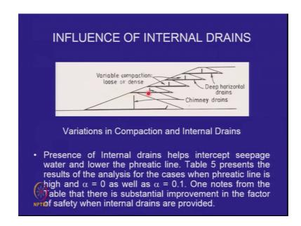
Can compaction prevent this failure, that is the question we are like to address 1.6 went to 1.9 when the ash is compacted that is very good, but 0.71 went only up to 0.82.
