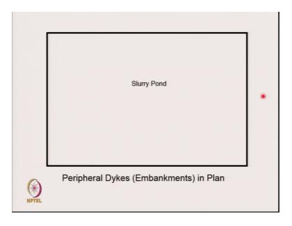
Critical to all this is the location of the decantation well and let me try and highlight this problem. This is the slurry pond. Let us say this is the area that is been given to us for the purpose of design of a slurry pond. And we are going to do upstream method of construction. So, I need to have two ponds. So, what I will do is I will bifurcate this into two so that one pond can be working another pond can be closed.
