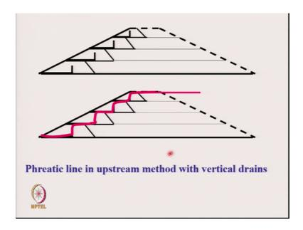
One thing which I talked about in the upstream method as we can see the internal drains are provided in each dyke; and consequently the phreatic line which develops is close to the downstream slope.
