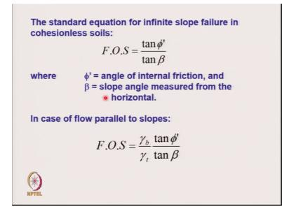
So, we looked at the fact that the factor of safety could be evaluated using the infinite slope failure methodology for the dry case and for the flow parallel to the slope case. And we said that the factor of safety when c dash is 0, becomes tan phi dash by tan beta and if there is flow parallel to the slope it becomes gamma b by gamma t tan phi dash by tan beta.
