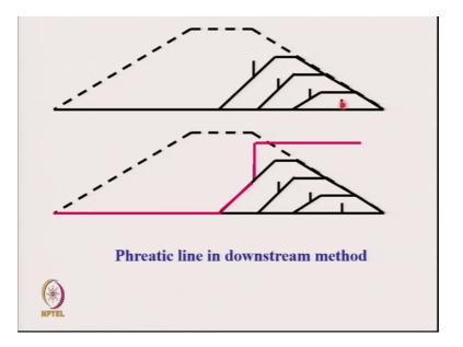
In contrast, in the downstream method of construction the drains are far away from the downstream slope, this is the final drain. Consequently, a phreatic line looks like this, bulk of the embankments is not saturated.
