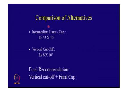
So, this was proposed. And in comparison to that one kilometer 1.6 kilometer by 6 hundred meter liner which was proposed was very expensive. The vertical cut off wall
