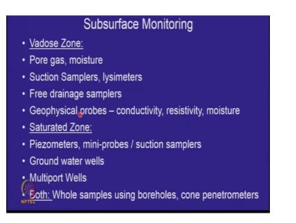
So, in this lecture and in the earlier lecture we are only been looking at monitoring of subsurface environment, when we looked at the subsurface environment we talked about the vadose zone which is a three phase media. And the saturated zone and we said the saturated zone is simpler because you just take out the groundwater and we want to assess the contaminants in the groundwater. It is so much more easier to take out the liquid than to take out the three phases.
