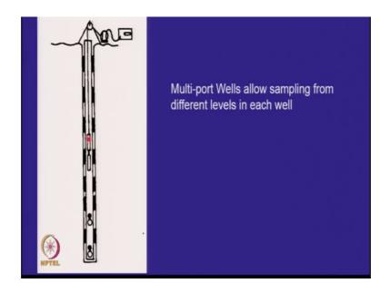
So, a multi ort device looks like this there is a particular type of sampler, we will not going to details of this, this can be a vacuum sampler or a numeric sampler.
