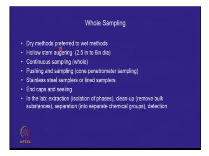
So, typically dry methods are offered do site investigations along coarse grades for hole samples using dry methods, hollow stem auguring. In soil mechanics we do SVT values, want once every 1.5 meter depth every 5 feet interval. Here instead go for continuous sampling that keep on just taking out samples, you do not have to measure any values you take what I say sample and you take out another sample, drill forward take another sampler.
