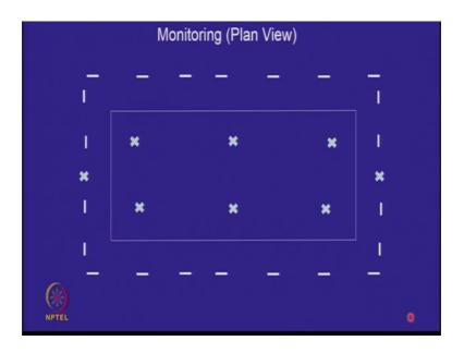
And that is to detect early, and to ensure that no contamination crosses the boundary of the landfill. In plan also we would be doing monitoring around the perimeter of the landfill and at various points above the landfill on the landfill surface and beneath the landfill.
