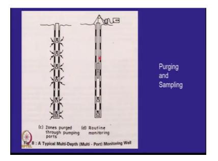
Install my device then I do the purging well development, I keep all the ports open and suck out the water what is the idea of doing this? All the bentonite slurry or drill fluid which we have put into the soil, first that will come out; well development takes weeks it does not get developed in a day.
