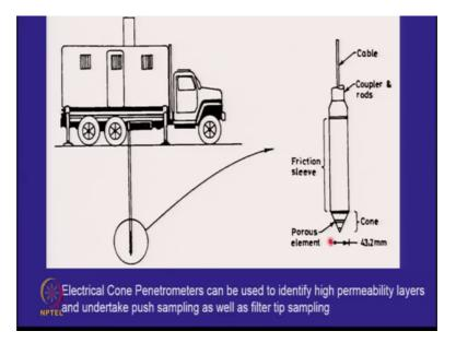
So, I will come back to this, but this is our traditional electrical cone penetration device, where a cone can be push down hydraulically into the soil.
