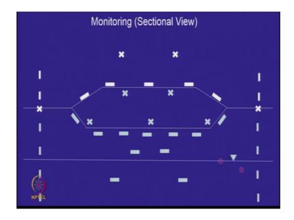
So, if you recall last time we talked about monitoring above the landfill, below the land fill and on the ground surface and on the surface of the landfill. We are basically focusing on how to monitor the environment beneath the landfill. (Refer Slide Time: 01:15)
