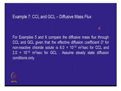
We have so far focused on advective mass flux; that means, due to difference in head. We can also look at diffuses mass flux. The diffuses mass flux requires us to use the Ficks Law and we have not gone into detail about the Ficks Law in a classes, but I will give you two formulae which we are going to use here and we are going to use parameter called the effective diffusion coefficient.
