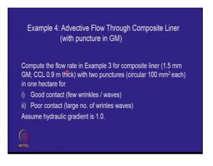
So, if I use the same geo membrane and the same compacted clay 1.5 mm thick geo membrane, 0.9 meter thick clay. Again two punctures in one hectare, then I have some empirical formulae for good contact and for poor contact if the hydraulic gradient is one.
