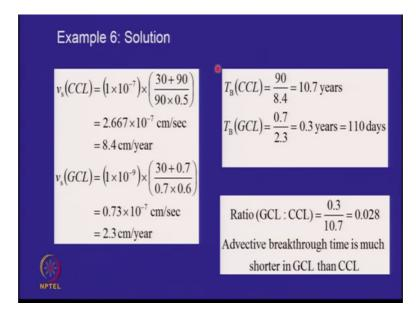
So, with this we can find out the break through time. So, let us first look at CCL in 10 to the power of minus 7 centimeters per second, 30 plus 90 over 90 into 0.5, this is the porosity effect and the seepage velocity will work out to be 8.4 centimeters per year. So, the important thing which I am trying to tell you is, Q is large; how much is the Q? 1 1 5 1 liters per hectare per year; the question is when does it start to come out in?
