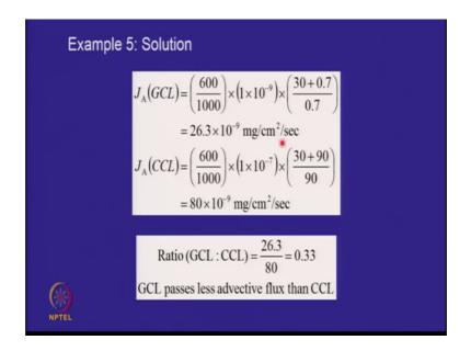
In the GCL, please note 10 to the power of minus 9 centimeters per second is the k. This has the 600 milligram per liter. So, we are trying to convert milligram per centimeter cube. So, 600 by a 1000, head is 30 centimeters, thickness is 0.7 centimeters and you should get this value of advective flux through GCL. Please confirm that you are getting this value. Anybody is confirming it?
