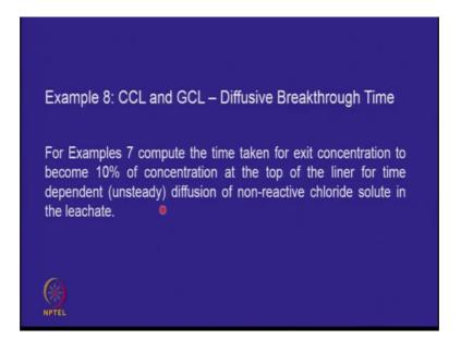
So, advective break through time was 10 years, 10, 11 years compacted clay liners and a few months in GCLs. To find out diffusive break through time it is little tricky, in the diffusion because you now have to use transient formulae, you have to use transient formula.
