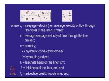
We know that v is equal to k i and v is called the average seepage velocity of the flow through the soil or through the liner. We first compute not the average seepage velocity, but the seepage velocity through the voids of the liner. So, v s is defined as the seepage velocity through the voids which is nothing, but v divided by porosity. So, I can get the value of v s, if I know the value of v s the leachate has to travel the length L. which is the thickness of the liner.
