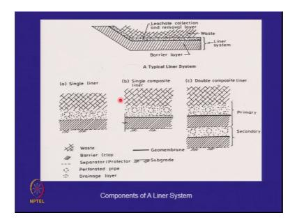
And let us go back to the liner system that we talked about. So, that is the this is a single composite liner the barrier layer the compacted clay the geo membrane and on top of that; that means, any leachate which comes to the side slope comes down and any leachate which comes there comes down and this is where it is collected.
