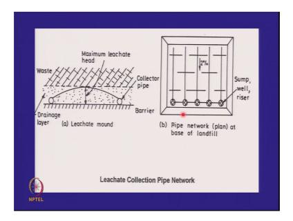
So, that the sand does not come and fill up the voids. So, this is a typical leachate collection trench and the base of a landfill.
