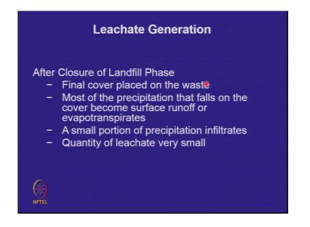
So, this is main thing. After the closure final cover is placed on the waste most of the precipitation becomes surface runoff or evapotranspiration. Small portion of precipitation infiltrates. And what that infiltrates again the internal drainage layer takes it away and quantity of leachate is very small. And I come back to this diagram, what I have put on the board.
