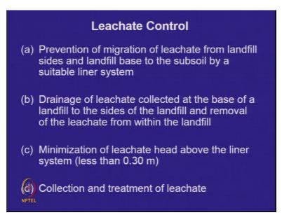
So, the next having kept the leachate to a minimum, leachate is still going to come out. So, what? So, how do we control this leachate? We have to take the leachate to the sides. The leachate should not point up into the center of the landfill. So, we first you have a liner which prevents this leachate from going down into the soil. Drainage of leachate collected at the base of a landfill to the sides of the landfill. And then removal of the leachate from the sides that is critical.
