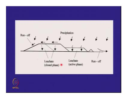
These are the closed phases this is the precipitation and that are the runoff. So, this will go to a surface water drain here. That is the active phase and what falls on it will give you the main leachate right. You have to have a bump here you do not want the water which is falling here to come here and start coming down. So, you have to prevent any water from any side coming into the waste.
