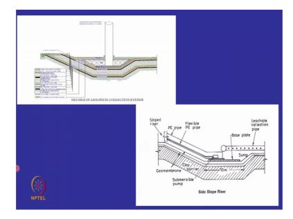
So, with this head these pipes must be equal to match the q which is coming down. If more q is coming down put more pipes; that means, you have to reduce the spacing of the pipes if less q is coming you can spread them out; typically, this pipe 50 to 75 meter spacing hundred meter spacing. And these are the 2 diagrams this is a vertical well. So, this is your sand drain.
