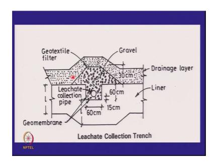
And again please understand that, this is the leachate collection pipe and it should be surrounded by gravel and the size of the gravel should be larger than the size of the perforations.
