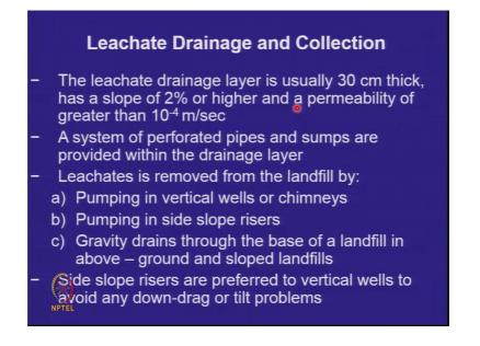
So, the leachate drainage layer is usually 30 centimeters thick has a slope of 2 percent or higher and a permeability of greater than 10 to the power of minus 4 meters per second, or greater than 2 to the 10 to the power of minus 2 centimeters per second a system of perforated pipes and sumps are provided within the drainage layer.
