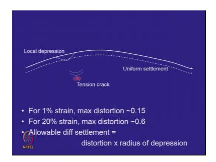
But the issue is if you have a local depression right if you have a local depression this is going to point up with water and please remember once you have a local depression you have a tension crack at the bottom right if it is flexible the tension crack will not form, but how flexible can you be. So, one of the indicators is in highly biodegradable wastes how much tensile strains can you can talk.
