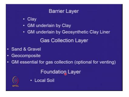
If the Geotextile; if the Geonet plus the Geotextile is available as one unit its one roll. So, the number of operations in installation goes down. So, that is a Geocomposite. So, I can use a Geonet overlying a geomembrane for drainage or I can use a Geocomposite and the same can apply to a gas collection layer the same can apply to a gas collection layer because gas will flow at a faster rate in a Geocomposite than water.
