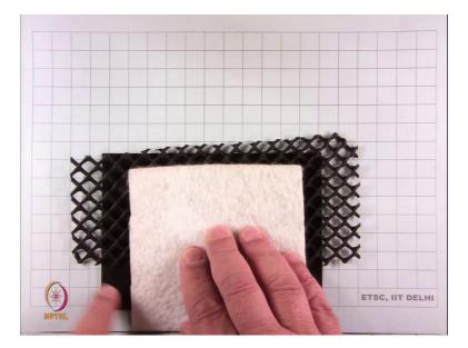
This I am bothered about the fact that fine should not come into this. So, what will I do to prevent fines I will put a separator. So, now, I have a material geomembrane at the bottom a Geonet at the top and filter Geotextile above it.
