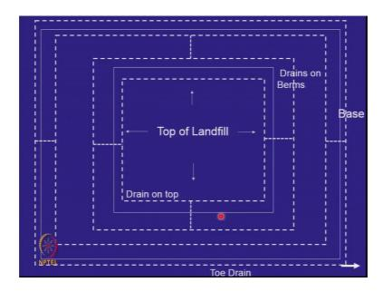
So, we should take care of the surface water very carefully if I look at a top of a landfill from aircraft or a drone; let us say this is the top of a landfill. So, what will you find 3 to 5 percent slope a drain here this captures all the water which is falling on the top these are the 2 berms. So, there is a drain here on the berm.
