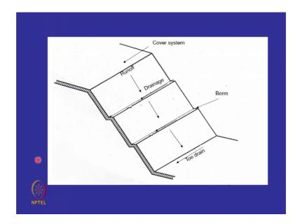
So, please see the arrangement you will have a diversion channel or an interceptor channel which should not allow the water to come on to the landfill whatever falls on top of this should go out from a drain here and a drain here and a drain at the berm and should go to the storm water drain at the toe and a better view allow the water to runoff down have a berm; down have a berm; down have a berm on the berm have a drain to collect the water.
