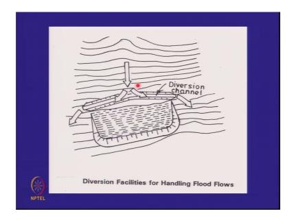
And this is the concept of the diversion channel or the intercepted drain if you are on a side slope landfill please catch the water and divert it from the sides do not let it enter the landfill.
