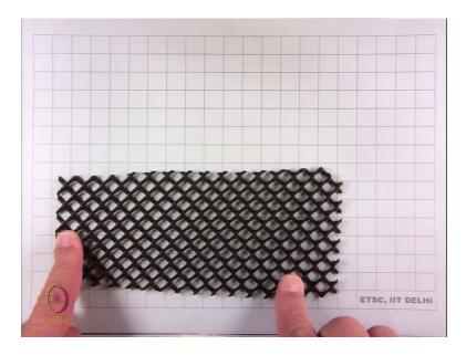
I am taking a geomembrane and putting this net on top can this net replace the sand that is the question the water will be percolating down from the surface layer and the protective layer into the drainage layer it will come and rest on the geomembrane.
