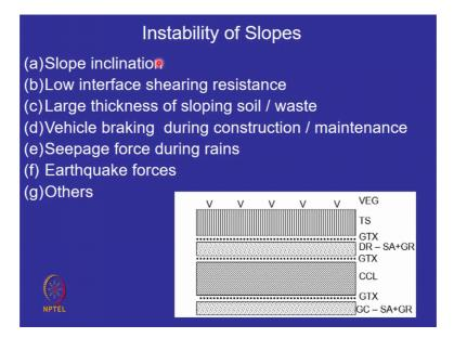
So, instability occurs because of slope inclination low interference interface shearing resistance no matter how rough I make my geomembrane it still is not having the highest phi dash large thickness of the soil on top vehicles will travel on this cover while you are making it seepage forces during rains earthquake forces will occur and others.
