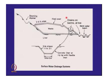
Which landfill is more affected by surface water above ground or side slope landfill the problem is the moment you have side slope landfills the water is coming down the slope it will tent to accumulate. So, as I said you have a 3 to 5 percent slope here and 3 to 5 percent slope here this slope which I am talking is at the top of the cover it is not the side slope the side slopes have a different value which we will talk about.
