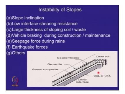
So, all these interfaces in fact, bentonite manufacturers will tell you that if you are going to make a slope steeper than 3 is to one you have to use the special bentonite which is got a special GCL which has got a reinforcement inside which does not allow failures to occur.
