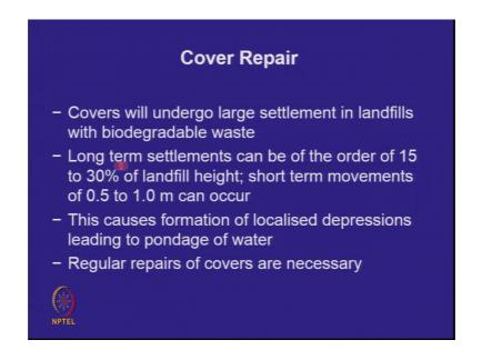
So, this is the way to repair covers. So, covers will undergo large settlements long term settlements can be of the order of 50 to 30 percent of landfill height short term movements of half to 1 meter. So, whenever you have a depression which is local see when I talk about 15; I am talking of the whole thing settling with time, but local depressions which form are typically half to 1 meter and these can cause bondage. So, regular repair is required.
