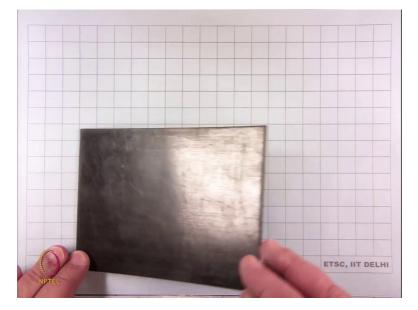
So, let us see starting with a geomembrane then a Geonet and then a Geocomposite. So, we all remember this smooth geomembrane and we also all remember rough geomembrane and this is going to become very important in covers.
