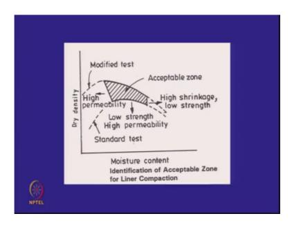
And we have to compact wet of optimum as I told you last time. And here you will be able to find out through your laboratory what is the additive content that you need for example, in Delhi silt we are adding bentonite clay. And you see about 5 percent clay is sufficient for getting the permeability that we need.
