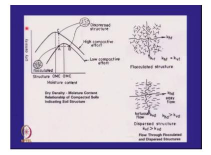
So, remember we go back to our standard compaction procedures; we go back to standard compaction procedures. And this is the light, proctor compaction test this is the heavy proctor compaction test. If you are compacting dry of optimum you are going to get a flocculated structure we all know this if you are compacting weight of optimum you are going to get a dispersed structure. When you have a dispersed structure your permeability is low.
