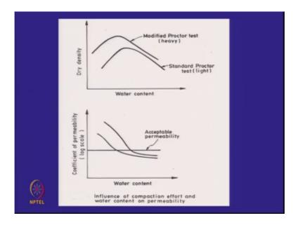
And these are not your standard falling head permeameters or constant head permeameters will do this in the next class. And we have to then work out how do I get the coefficient of permeability below the acceptable level.
