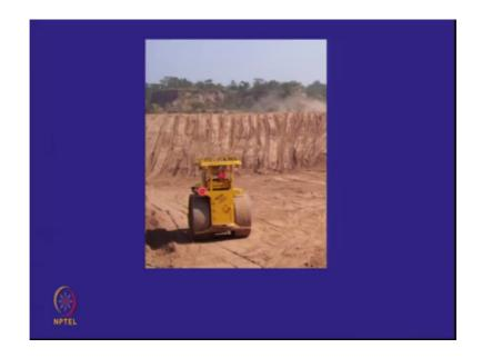
And we are now compacting it. This is not that a roller you should be using what type of rollers do you use in clays.
