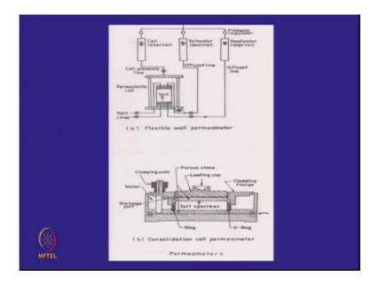
And we have to use some laboratory testing devices for finding the permeability of clay, because we have to assure this 10 to the power of minus 7 centimeters per second.
