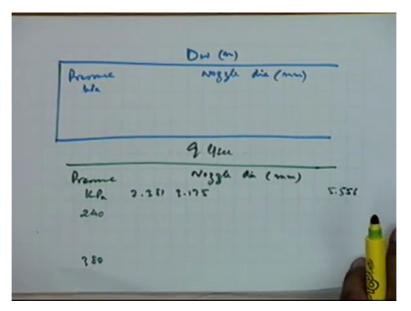
For example there is a table which gives the wetted diameter in meters for different under different pressure the nozzles of different diameter so for different nozzles running under different pressures you have their wetted diameter, how the wetted diameter varies because if you want to select a wetted diameter which is which is a desirable wetted diameter you can use this table.
