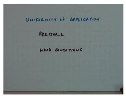
The last class we had started looking at the uniformity of application and we had mentioned that the uniformity of application is dependent two aspects, is highly influenced by the pressures which are the prevailing pressures in the network of the sprinkler irrigation system and the wind conditions which are the natural conditions. So these two are the factors which influence the uniformity to a large extent. (Refer Slide Time: 1:50)
