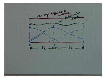
Similarly on the, on a lateral line you might have, these are the three sprinkler positions. That means this is a 0 level for these three individual sprinkler heads. And each one has its own pattern. So if the pattern of this is somewhat like this, pattern of this one is the portion which is influencing up to this area. Similarly on this side if this is the portion which is influencing to this area.
