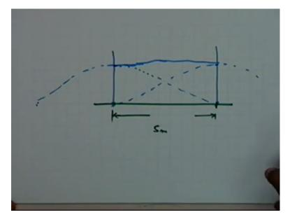
If we draw the same thing in terms of, in one section let us say that if is the spacing between the laterals which is the main line spacing, on this case you have one lateral here, the other lateral here and you will have some sprinkler nozzle at this level because all these sprinkler nozzles will be in the same line. So the pattern of the individual sprinkler nozzle is somewhere like this and similarly the pattern of the other sprinkler nozzle is somewhere, somewhat like this.
