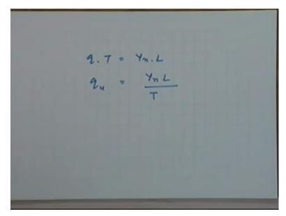
I can use this water balance or these two should match. Basically these two quantities should match. So you can say that q into T should be equal to your Yn into L. This is the first design criteria. This is the first design criteria which you can take, which you can consider. And you can find out now, you have found a relationship between the two, you can find out any quantity knowing the other set of quantities. Now here comes a decision what you know and what you want to find out.
