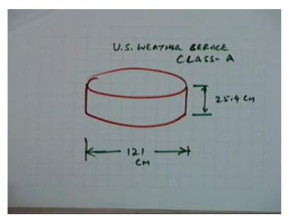
Now what you do is that you fill this with water and the depth up to which you normally fill the water, this depth should be maintained in such a way that the fluctuations are within around 5 to 7 point 5 centimetres. From the rim of the Pan you can go maximum up to around
