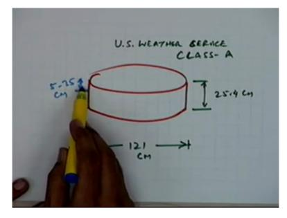
The other requirements are, there are some requirements for placing this Pan that it should be placed on some platform, that can be a wooden platform on which you can place this so that there is lot of air which is passing through and the ground surface temperature is not affecting the temperature of the water. But there are different types of Pans.
