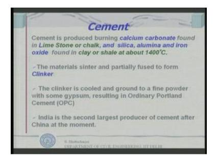
So, let us look at cement composition now we mentioned earlier it was in the last module sometime. We said that cement is produced by burning calcium carbonate found in lime stone or chalk and silica alumina and iron oxide found in clay or shale at about 1400 degree centigrade.
