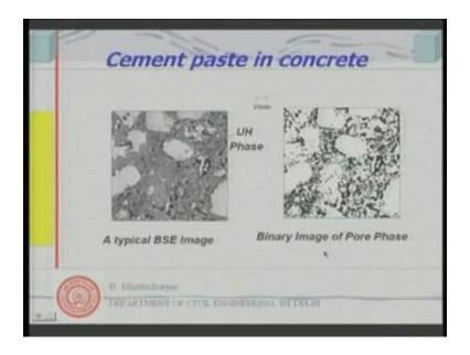
So, this is the strength you know we can see the c 2 s and the c 3 s main strength you can perform. Now, if I look at the back scattered electron image of cement paste in concrete this is how it would look. You see back scattered electron. So, therefore, from the places where electron does not scatter back they will look black in a back scattered electron image you know electron microscope image. Actually, the black ones are the pores the
