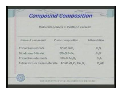
Then I get this is again showing the same tri calcium silicate to remember it because this is a long name tri calcium silicate, di calcium silicate, tri calcium aluminate, tetra calcium alumino ferrite has been repeated. So, this is clearly remembered because that is the terminology one uses again and again in the context of concrete and cement right.
