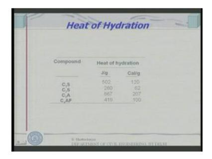
If you see the relative heat produced by different compounds we will see that c 3 s produces about 500 and 2 joules per gram it should be and this is 120 calorie per gram. This should be joules per kg this should be joules per kg c 2 s produces 260 c 3 a produces 867 and c 4 af produces 419. So, this is the relative heat of hydration and this produces maximum heat of hydration. It generates maximum heat on reaction where as this generates least this is the next and so o so forth.
