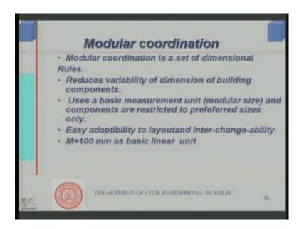
Modular coordination is nothing, but it is a set of dimension or rules and it reduces the variability of dimension of building components. So, what you do you have a basic unit, basic module and everything is repetitive. So, your layout will also be modular layout so that, you can use one part one component, you know you can use interchangeably the components building components.
