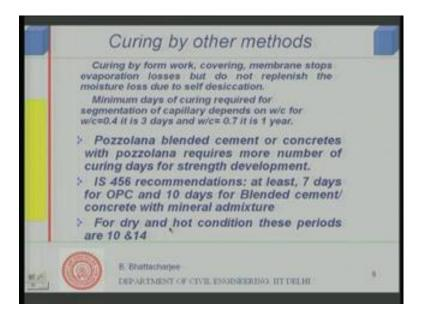
I mentioned to you curing by form work; covering with membranes and you know all this would actually covering form work and covering with the membranes etcetera, covering with you know this covering membranes form work, all this actually stops evaporation loss, but do not replenish the moisture loss due to self desiccation. So, they can be as good as the moist here right. So, that is I have mentioned already and explained.
