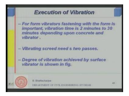
For form vibrators fastening with the form is very very important vibration time is about 2 minutes to about 30 minutes depending upon concrete and the vibrator. So, here you require longer vibration longer period of vibration depending upon of course, the situation, but it should be firmly held in position. Because, if it is not firm then there will be some energy loss at the junction also.
