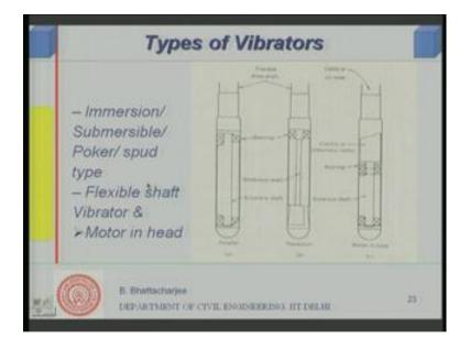
So, let us see 1 by 1, first we will look into internal vibrators continue with the type of vibratos; these are called immersion, submersible, poker or spud type vibrator. They are either called immersion, submersible, poker, spud type this is first 1 is the flexible shaft vibrator and the other is a mortar in head. Now, you can see this diagram this is the flexible drive type and this is mortar in head itself this is a right.
