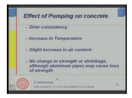
Well, practically there is no negative effect; it becomes makes it a little bit drier after all you are applying pressure to the concrete. Then increase the temperature slightly, air content in the concrete may increase well again and as far as strength shrinkage etcetera are concerned. There is no negative effect; no reduction in strength, no reduction, no increase in the shrinkage takes place.
