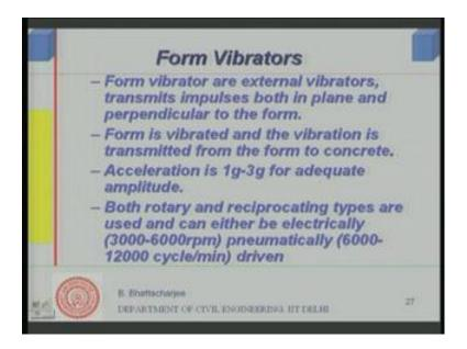
The other variety is the form vibrator, these are used these are actually external vibrators and these transmit pulses both in plane and perpendicular to the form also. In other words, you place it on to the form itself and it vibrates the form and when it vibrates the form, in turn vibration of the form is transmitted to the concrete and causes concrete to vibrate. Naturally some amount of energy is lost in the process, because your vibrating in the form also right.
