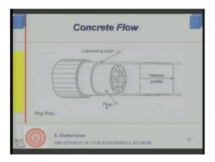
Now, the flow would look like these plug flows as you call you see you have a fine lubricating layer at the boundary. Fine lubricating layer this is the plug you know complete plug, which is solid and this lubricating thin layer the velocity gradient exist here and for this whole plug the velocity is constant. So, velocity profile if you look at it is constant throughout and here there is a variation of velocity 0 at the boundary and there is an implicit.
