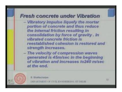
When you supply vibratory impulse you know this liquefy the mortar portion of the concrete and reduces the internal friction; basically what is happening is you know, you
