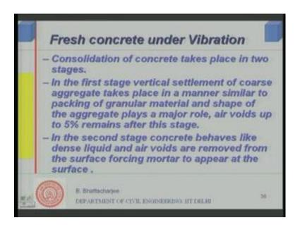
Compaction takes place in 2 stages: in the first stage vertical settlement of coarse aggregate takes place, in a manner similar to packing of granular material and shape of the aggregate plays a major role, air voids up to 5 percent remains after this stage. So,
