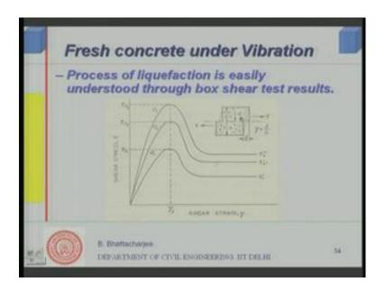
This is easily understood, 1 can do what is known as box shear test and early work done in box shear test. You know here what is done is you have a concrete here and you have a concrete here. These are all fresh concrete sort of fresh just after mixing all that it does not solidify. So, you have apply pressure here I mean force here and force here, the shear force here; within 2 boxes this is a box mould it is usually done for soil.
