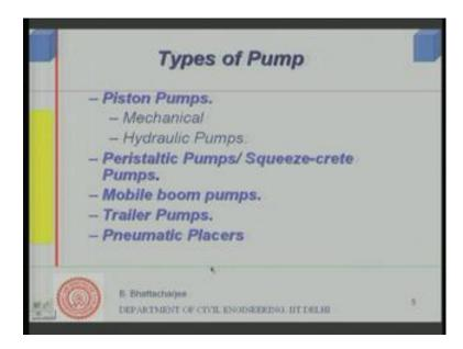
There are varieties of pumps, so if we look at types of pumps: the first ones are the Piston Pumps: Mechanical and Hydraulic pumps, your second variety is called Peristaltic Pumps or Squeeze Crete Pumps. Well same, either this piston pumps they can again be Mobile boom pumps, can be Trailer Mounted Pumps and there can be other type of pneumatic placers of concrete.
