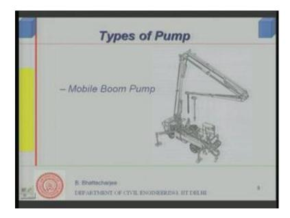
And same any one of these types of pumps can be actually mounted on a truck, so it is a mobile boom pump.
