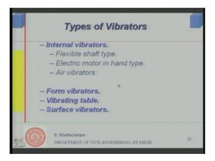
Let us see what are the types of vibrators there is something called Internal vibrators the most popular 1s and many of you might have seen it, if you seen a construction side usually they are 2 types: Flexible shaft types which are the most common type and electric mortar in hand type. Then, there are Air vibrators that are again internal vibrator air vibrators. Form vibrators those vibrates the form itself, then vibrating table, surface vibrators.
