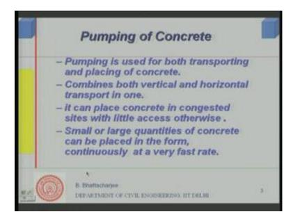
Let us see first what is pumping of concrete? Pumping is used for both transporting and placing of concrete. Well this combines both vertical and horizontal transport in 1. So, it's quite volatile in that sense it can place concrete in a very congested site with little access otherwise. And small or large quantities of concrete can be placed in the form, directly continuously at a very fast rate.
