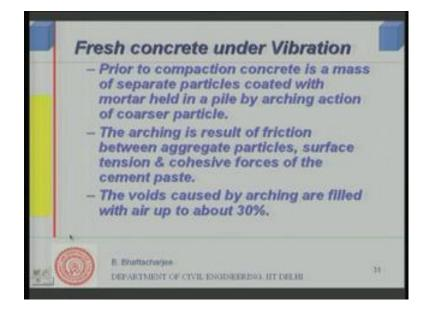
Before compaction it is a mass of particle essentially you know if you have essentially particle at system, something like this heap of particle of various sizes just there you know supported 1 after 1 over another. Sort of an arching action it supports you know it's like soil, which you can have heap of soil, so it's like that concrete masses. So, this has particle separated and coated with mortar held in a pipe and that is called arching action of the coarser particle.
