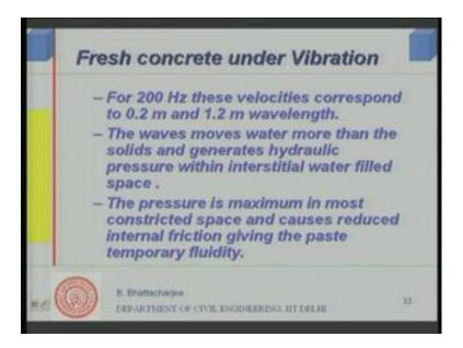
For 200 hertz this velocity corresponds to 2 meter and 1.2 meter wavelength. Because, velocity is know and you know v equal to f lambda, so if you know the frequency 200 hertz corresponding wavelength we can find out. These waves actually causes movement
