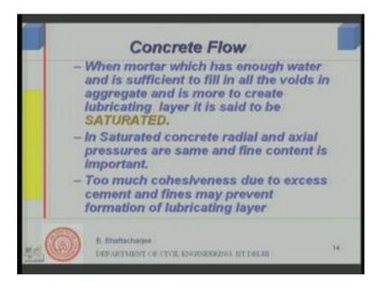
So, this is what we call it plug flow now, this is facilitated when concrete is what is called Saturated. What is state of saturation? When mortar in concrete has got sufficient water and that can feel all the voids in the mortar system. And the mortar itself fills all the aggregates and slightly more may be and the system is such that, it can create you know sufficient cement paste in the mortar system.
