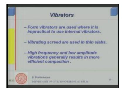
Form vibrators are used where it is impractical to use internal vibrators I have already mentioned this. Screeds are used in thin slabs so, because you can put it on to the surface and vibrate it may be floors know flooring. High frequency and low amplitude vibration generally results in more efficient compaction, so high frequency low amplitude that is the idea. Now, let us see what happens when you subject fresh concrete you know to vibration.
