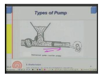
Continuing with the type of pumps this is what a piston pumps look like, see it's is a reciprocating pump as can be seen and currently this 1 is in its suctions probe where by concrete is through the suction hopper, concrete is concrete enters into the pump. This piston moves along this direction and you see along the suction direction this moves like this. And this valve now it is at open position, whereas this valve now is at closed position.
