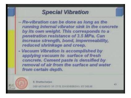
So, let us go back and see something about special vibration some time I might do revibrations, but so long my needle can penetrate into the concrete re-vibration is there is no problem my needle must sink into the concrete right. So, this corresponds to a penetration resistance of 3.5 MPa now, penetration resistance is a test for measurement of concrete setting.
