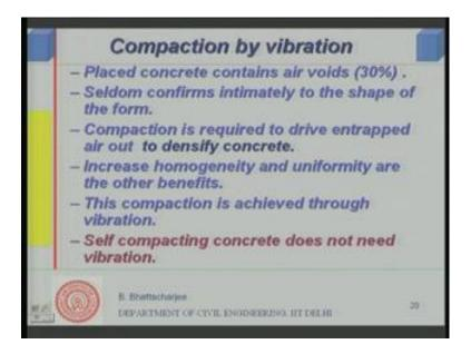
Now, let us look into next phase of our production process that is called compaction. And this compaction we will do usually by vibration, but not in all cases, the special cases will come. This is required, because in placed concrete you place through whatever means normal concrete will contain will contain large amount of voids as much as 30 percent. And of course, you do not place exactly into the shape unless highly flow able component that is a different issue altogether.
