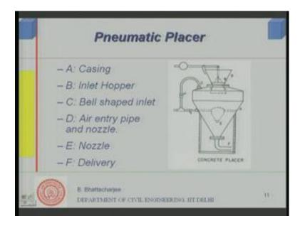
The pneumatic placers is used for a grouts usually as you can see it has got a casing this is the casing, this is the inlet hopper, this is a bell shaped inlet and this is air entry pipe with a nozzle, this is also the nozzle and this is the delivery. The concrete is actually driven by compressed air pneumatically.
