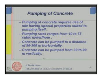
Now, let us see what is the basically is there any difference of the mix required for pumping. Well that is there is the mix that we can transport through pumps, require some special properties ranges of pumping rate can be 10 to 75 cubic meter per hour and concrete can be pumped through height of 90 to 300 meter horizontally.
