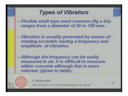
Here, this is the most common and its diameter ranges from 20 to 180 millimeter, usually generated by means of rotating eccentric having a frequency and amplitude of vibration that you have mentioned. And the frequency can be this we have already said right and more about this we will have in a table.
