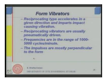
Reciprocating type accelerates in a given direction and imparts causing vibration. So, basically imparts an impact and as I said, it is both plane in plane that is along the plane of the shattering and also transfers direction of vibration is important on to the concrete. So, it vibrates you know transfers both impact energy transmitted horizontally also vertically along the plane of the form wall and also to the concrete directly.
