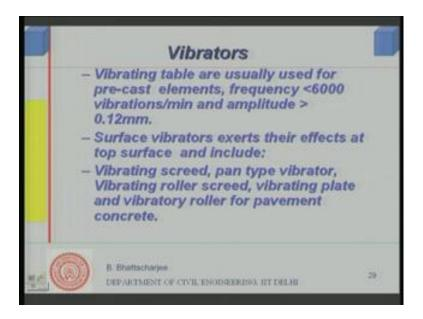
Vibrating table, so form vibrator we have discussed internal vibrator or needle vibrator; the other type of vibrator is a vibrating table. Vibrating tables are usually used for pre cast elements like you might have seen if you have gone to a laboratory, where concrete cube are tasked for testing purposes there this is a vibrator on a table. So, table vibrators are damn used only for pre cast elements, because large slab pre cast slabs we will discuss what is pre cast later on.
