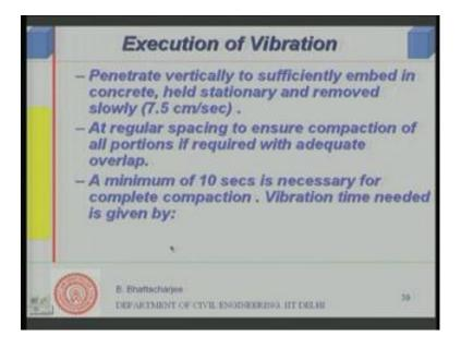
Well this is while executing vibration the needles vibrators are penetrated vertically to sufficiently embed into the concrete, then held stationary and then removes slowly at a speed of about 7.5 centimeter per second. So, that would be the best way of vibration you have to ensure a regular spacing that compaction of all portion. If required there can be adequate overlap you know I can show you diagrammatically something like this.
