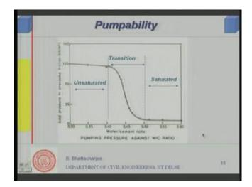
So, pump ability is governed by what? Lubricating layer must be brought the saturated concrete is easy to pump. And early experiment done in 1950s have shown that water to cement or rather you can say the fines ratio. The fines may include today, including fly ash and other materials which I mention which has cement ratio fine in nature you know total powder fine very fine powder.
