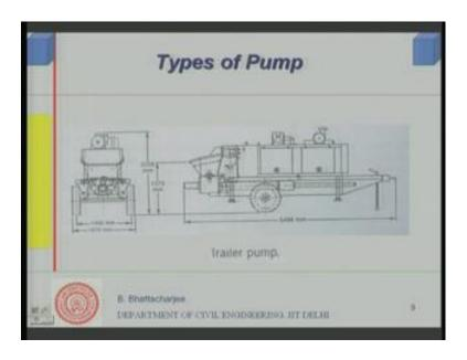
This is a trailer mounted pump as you can see, the pump is mounted on the trailer and is very common. And usually used for large capacity pumps and that is what is mostly used currently in the country.
