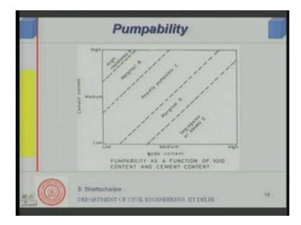
A little bit this you can see that when the total void content in the system versus cement content to the plot, void content it means that in void content the aggregate system overall and the cement content if you see. If you have high voids there will be segregation, because water will be just move away leaving the solids. So, the tendency to segregate or bleed when your high voids in the medium you have less amount of fines.
