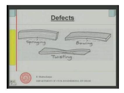
And other defects are twisting, bowing, springing; all these defects are possible in timber after sawing and seasoning.
