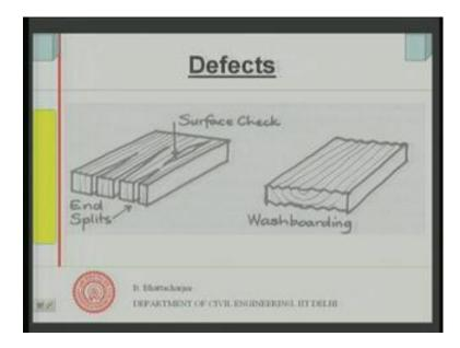
For example, end splits; you know like this 1 end splits, as shown surface cracks are forming, then this wash boarding something like this right.
