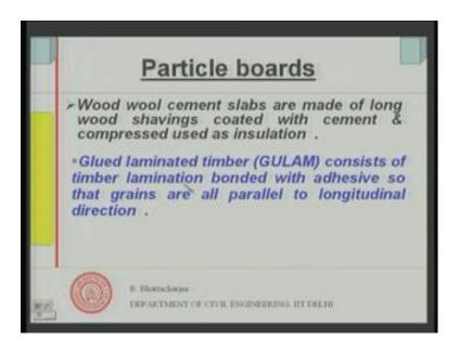
I said that cement is cement can be used for bonding purposes like particle boards can be manufactured with cement So, we have same cement you know in sort of cement mortar preparation, you essentially use sand. Now instead of sand supposing I am using wood shavings wood sawdust and all that. Therefore I can get the I can make it you know in
