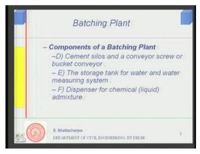
And next one is, of course, cement silos where I store cement and a conveyor, screw conveyor or bucket conveyor through which I actually transport the cement from the silos to the weighing device balance, and then of course, to the mixture. And then, followed by this would be the storage tank for water and also water measuring system, right.
