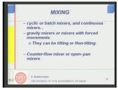
The mixer type, if I look at it, there are cyclic or batch mixers, as I mentioned, because conventionally what we see are cyclic or batch mixtures. It mix, takes one batch at a time,
