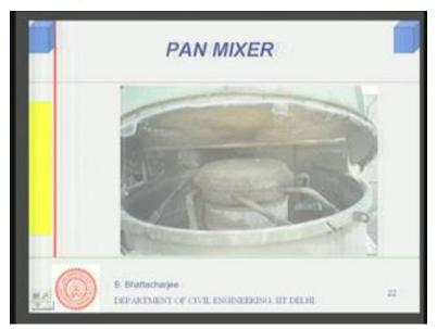
A pan mixer will look like this. It is flat, you know, it is not gravity type, it is fixed mixer and you have blades like this and blades like this. Some are in the outer periphery, some are the inner. The pan drum, this drum rotates the blades in the position or they can have counter flow, they can have a counter flow, relatively they must, the drum and this blades, drum and the pan, they must move in the opposite direction, so as the material would be moving, let us say, in this direction.
