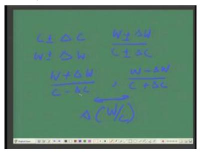
I will get, you know delta C is the variation in cement content and delta W is the variation in water content. So, my actual cement it should have been seen C, so plus minus delta W by C and water actually, originally, was W. Now, my error in measurement is delta W, so my water cement ratio will now become this plus minus delta W by C plus minus delta C. So, the range of water cement ratios I can write like this. The
