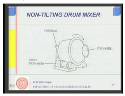
The other is non-tilting type of drum mixer where it is fixed, it does not tilt. So, you have charging hopper on this side and there are, in this one this blades or baffles are there, which lift up the aggregate. As I said, this is non-tilting.
