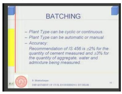
So, this is what batching plant looks like; this is what batching plant. There can be two types of operation possible for batching plants, one could be cyclic type, other is continuous. One I showed was actually a cyclic type; one I was showed is cyclic type.
