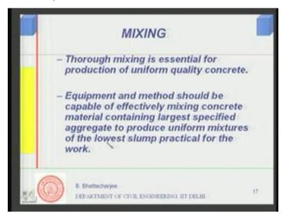
Now, we can look into mixing, the other process, other important process. We have weighed the material, then we got to mix it, the hand mixing is not possible in large jobs, anyway. But even in small job, hand mixing cannot give you a good product. So, mixing
