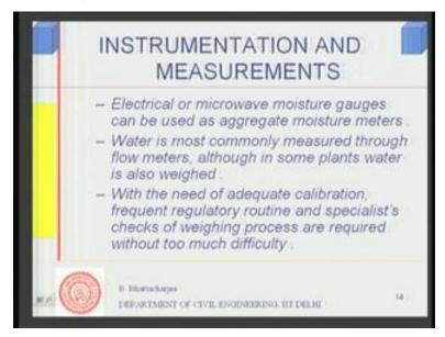
Moisture measurement of aggregate is very, very important. You do not want, of course, cement to get contaminated due to water, that is why, we store them in silos. But when it comes to aggregate, you store them in open. So, if there are rain or due to relative humidity particularly, of course, is mainly of rain or something moisture coming from the environment, so it can absorb some amount of moisture and this moisture needs a kind of correction in the batching.
