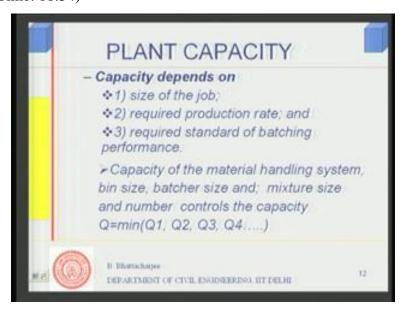
Plant capacity will depend upon the size of the job, what is the size of the job. If it is the small job, then you can use the small capacity plants, manual type. But if it is the large job, one has to use a large batching plant, mostly automatic type.
