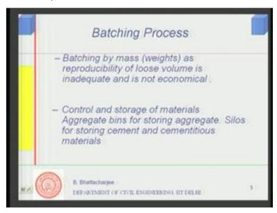
Why it is so? The reason is very simple. Since we want to mix the material in correct proportion, as we have designed it, therefore volumetric batching is not desirable because volume, the mix design is on the basis of mass. And volume of such particulate system depends upon the packing. If it is a lose packing, it will occupy more volume because the bulk density will be less. If it is a compact packing, its bulk density will be more and occupy less volume.
