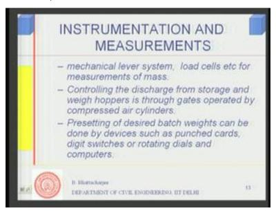
What are the types of instrument we use? Mechanical lever system, I just mentioned, that it could be mechanical lever system for weighing. Then, those are basically meant for manual, manual type of batching plant.
