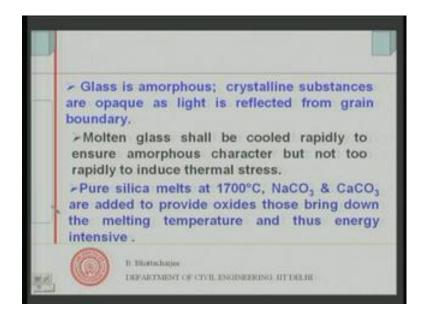
Glass is amorphous and we know that crystalline substances are opaque, you know if you look at the nature of the glass; glass is amorphous and we know that the crystalline substances are crystalline substances are opaque, because light gets reflected from the grain boundaries right. They are very compact and compact structure basically and regular arrangement of atoms. And at the grain boundaries light will get reflected. Therefore, they are all opaque right, whereas glass is not so right.
