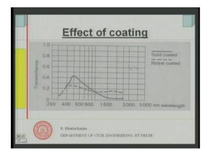
If you see effect of coating; gold coated have got this is again this is the visible range, this is where is the visible range, this is the infrared region gold coated has got high absorptivity here, but very low absorptivity where as at the higher side, nickel coated is something like this. Photochromatic glasses you know which is sensitive to the light, it actually the transmittance varies with the amount of light. So, it is actually photosensitive
