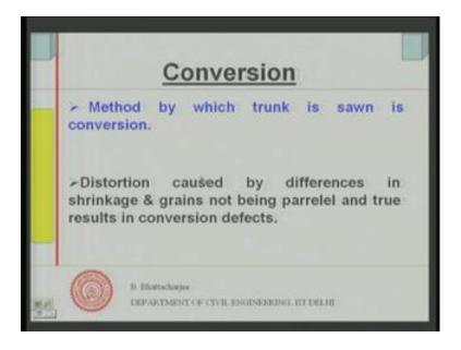
Now we have something called conversion; method by which actually trunk is sawn is called conversion. You have got 2 you have the trunk and you have to cut it into pieces, you have got it to cut into pieces in order to cut it into pieces in order to make timber out
