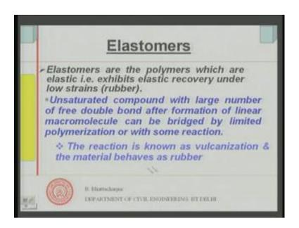
A third type of polymer is known as a elastomers and we have usage of all of them in civil engineering, you have thermoplastics and thermo sets will shall discuss detail them in detail some time later on. And elastomers you must a hard of them, because most of the bridge bearings; bearings in the bridge structure, bearing of the deck system over the period is usually elastomers.
