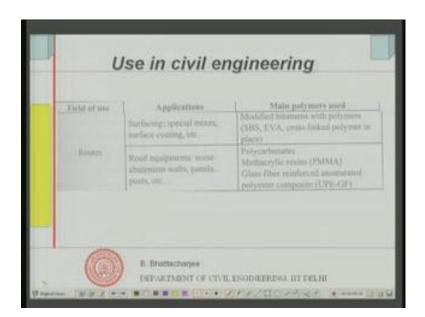
The second important usage of polymeric material is in roads for purpose of surfacing, because bitumen you know bitumen again is involved in is in it organic polymeric material.So, special mixtures surface coating extra for roads and modified bitumen with polymers extra.So, this is polymer in a modifier or modifier for bitumen system this is very common and this is where it is using roads.
