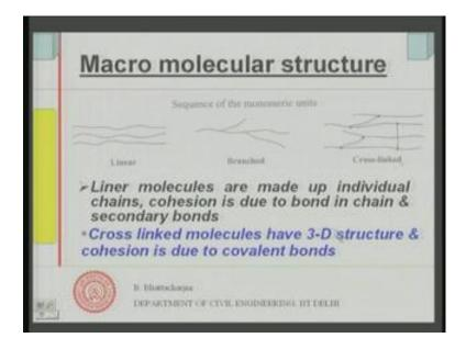
Let us see what is the macro molecular structure right? What is the structure of the macro molecule? We have seen the structure of course, other materials as such and this have what is called 3 varieties of you know monomeric units are connected. For example, in linear this will have call connected in linear manner in this 1, so this is called linear sequence of units they will be linear-linear structure.
