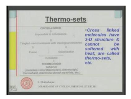
As suppose to this the cross link structure you know, if you see that in that case the sliding of the chains are not possible 1 over another and they are cross link. So very easily you cannot break, because there will be opposition from the cross link 1. So, there it is not easily you cannot separate or individualize the molecules so easily.
