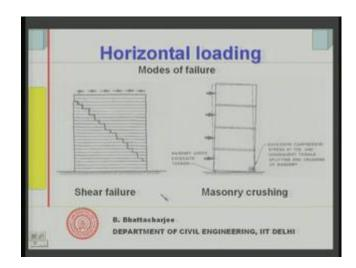
See what are the kinds of modes of failure? Under shear if you have shear failure it can show you know the shear effects will there is a shear force here. This can result in this can results in crack formation like this you know this is trying to it will separate out somewhere. So, diagonal cracking we would see. We will see diagonal cracking.
