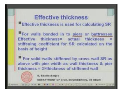
Now, one more issue we did not pick up earlier related to the load resistance to load of resistance to load of masonry structures effective thickness. Now, when we have, when you have strengthening of the wall through let us say: cross walls like cross walls or by piers or buttresses then the resistances against is provided by supports right. Hence what is done, what we do?
