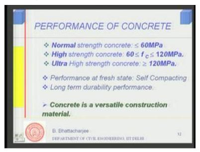
So, strength is one criteria and I said, normal strength concrete is 60 MPa. So, high strength concrete we define as one, which got 60 to 120 MPa cube strength. And ultrahigh strength concrete will be greater than 120 MPa. Now, strength is one criteria, but since we make concrete in its plastic state and then it hardens. And then it, actually its long term properties are also important. It should be durable, therefore we talked sometimes in terms of performance of concrete.
