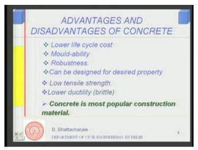
First of all, ordinary concrete, it uses stones and major volume of it is actually stones and naturally available sand or crushed stone, again, which are naturally available, thereby it is cheap. So, it will have low cost of production. First of all, cement is the costliest material among all of it, but then, cement paste, as we have seen, occupies only 25 to about maximum 40 percent in some special concrete, rest all is naturally available material. Therefore, it is cheap to produce.
