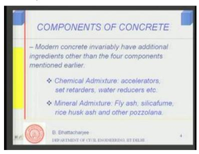
So, components of concrete, therefore cement and water, which reacts together and binds the aggregate. The aggregates are nothing but sand and stones, but this is not all. The modern concrete system also uses some sort of admixtures, as you call them, some sort of additional materials, construction chemicals, which when added to the cement system, actually improves its property.
