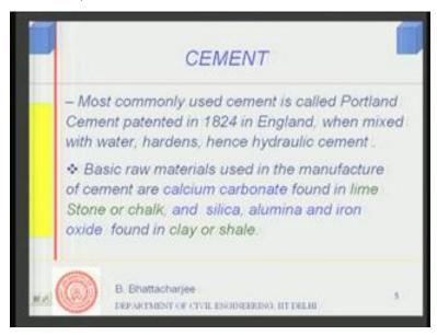
The most commonly used cement, we call it as Portland cement. It was patented in 1824 in England and this mixed with water hardens. And since it mixes with water and hardens, we call it hydraulic cement. Now, there are, that means, there are other kind of cement also, which need not be cementing material, may be, which need not use water. So, hydraulic cement is of this type.
