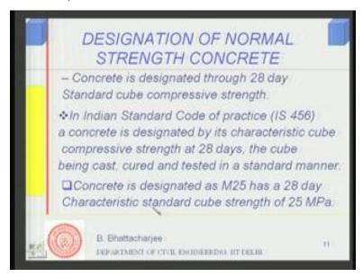
Now, this is, so far I have talked about concrete and cement composites, now let us come back to our most common material, that is, ordinary concrete, in general, concrete. Although I have talked about concrete and cement based composites, which have got wide range of properties and wide range of application also the most commonly used composites, cement based composites is ordinary concrete. This ordinary concrete strength ranges less than 60 MPa. We shall see this later on.
