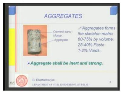
The second in component is aggregates, which forms the skeleton. These aggregates are nothing but stone, natural stone, either broken down or crushed to form the right kind of sizes that we require in case of, for making concrete, or they can be rounded stones as available naturally, say gravels. So, they are naturally available, but most often we use crushed aggregate depending upon the availability.
