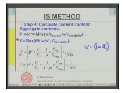
So, then next what I can do; since I know the water cement ratio and I know the water content, I should be able to find out water cement ratio first of all you know, first of all I must find out, what is the correct water cement ratio. And this is found out, as the minimum of water cement ratio from the curves that, I have mentioned and the water cement ratio for durability and then cement content, then I find out because I know the total water content.
