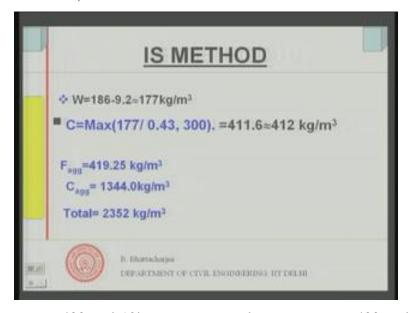
I have got cement as 400 and 12k g per meter cube aggregate as 400 and 19.25kg per meter cube coarse aggregate as 13.440kg per meter cube. The sum total therefore would
