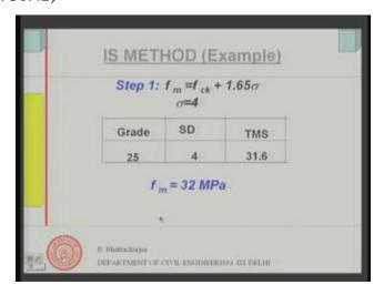
So, first step what we do; I said my grade is you know, first step is to find out target means strength. So, fm is given as fck plus 1.65 sigma and if you remember, if you recall I said that, for M25 grade of concrete 10 to 15; we use 3.5 sigma equals when nothing, is available. And from 20 to 35 possibly we use 25; we use or 25 to 30 we use for and above that we use 5 MPA. So, 4 MPA is a standard deviation given my grade is M25 that is known to me.
