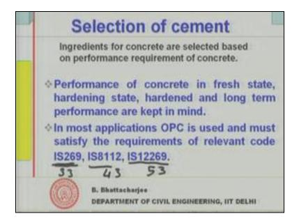
So, ingredients of concrete are selected based on performance requirement of concrete like cement also you select based on what is the performance requirement of concrete. What do you want from the concrete? And as we have mentioned earlier several times; Performance of concrete in fresh state that is this hardening state hardened state and long term performance are kept in mind. So, we select cement based on all this because you know we have seen earlier.
