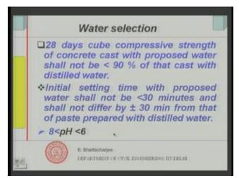
We actually compare 28 days cube compressive strength and you know strength of concrete cast with proposed water and that with the distilled water and the 28 strength should not be, you know it should be it should not be distilled water.
