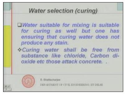
So, that is these are the these are the requirements as far as water is concerned as far as water is concerned curing water suitable for mixing is suitable for curing as well. It is suitable for curing as well, but 1 has 1 has to ensure that, curing water does not produce any stain same problem curing water of course will not affect the initial hydration process, but it can surely affect the long term durability.
