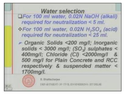
You need the sodium hydroxide 0.02 normal. You know you take 100 milliliter of water. The amount of sodium hydroxide needed to neutralize this 100 milliliter of water. We use 0.02 normal sodium hydroxide solution and this should not be more than 5 milliliter.
